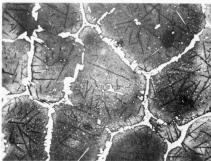
Figure 19. Ti-Ta-C: 35/61/4, Quenched from 2480°C
