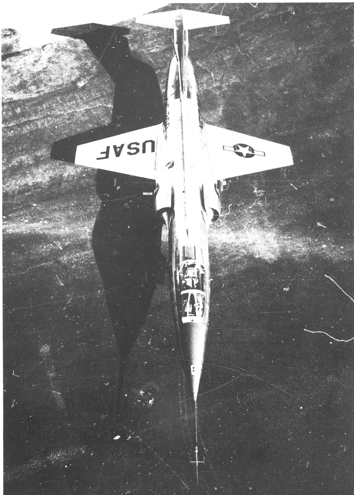
TOP VIEW OF NF-104A SHOWING NOSE BOOM INSTALLATION, RCS MOTORS, J79 ENGINE INLET CONES, 2 ft WINGTIP EXTENSIONS AND ROCKET ENGINE INSTALLATION.
