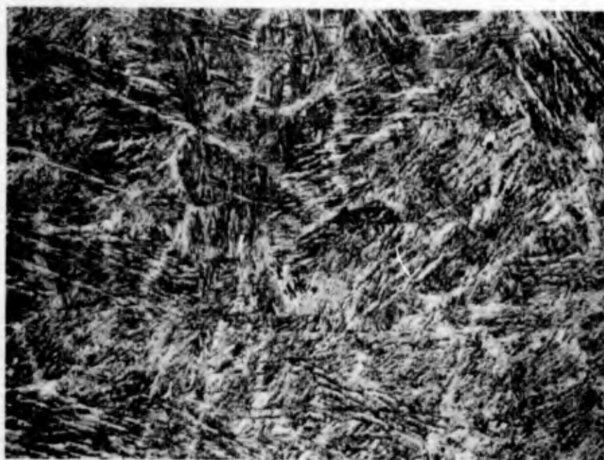
(a) Argon Shielded Weld P319 500X
