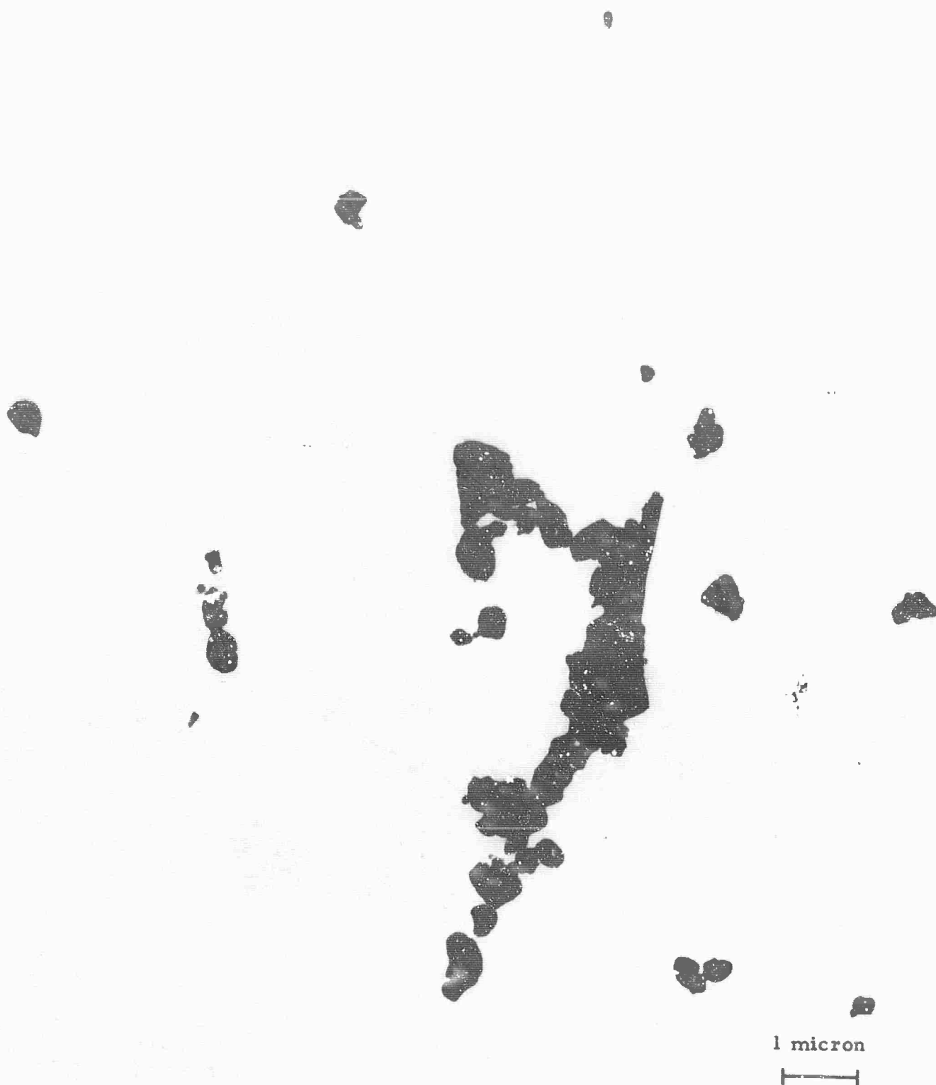
Fig. 10 Electron micrograph of an epoxy resin comminuted 72 hours at room temperature in the cryogenic ball mill (magnification is 15000X). The presence of small particles (0.2 microns) is shown. Similarly, the loose agglomeration of the small particles can be seen in this micrograph.
