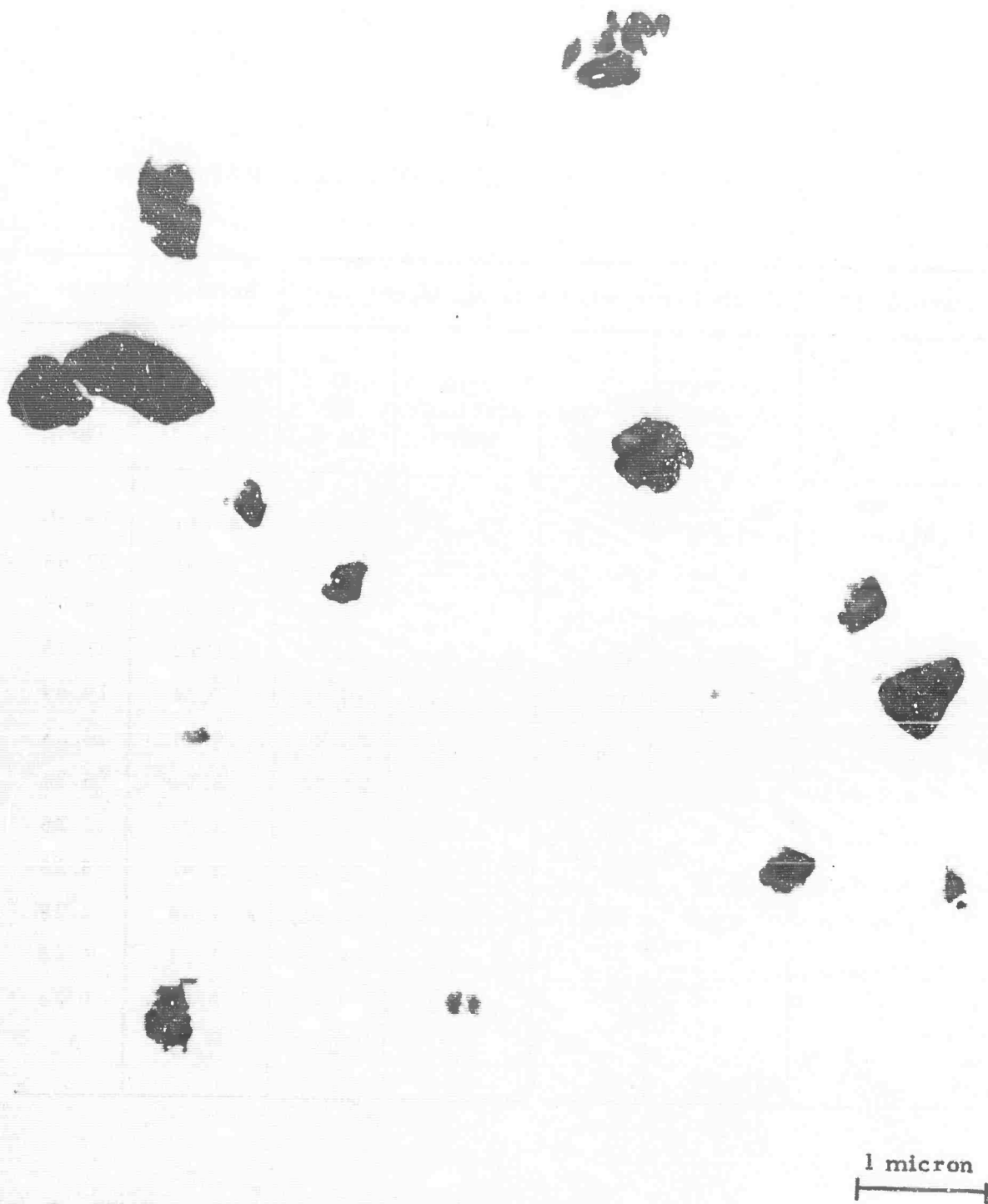
Fig. 7 Electron micrograph of glass-filled phenolic graphite at a magnification of 22000X. The very small particle size is shown, as is the presence of two phases. The statistical particle size analysis based upon this photograph and eleven others is presented in Fig. 8 and 9.
