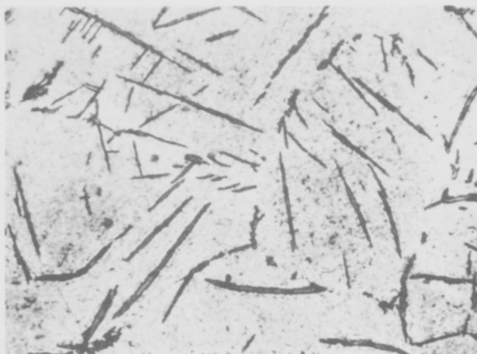
Figure 35. Zr-Ta-C: (60/38/2), Quenched from 2000°C. X1000 Apparent Eutectic Structure.
