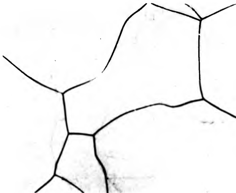
Figure 37. Zr-Ta-C: (55/5/40), Quenched from 3390°C. X1000 Single Phase Monocarbide.
