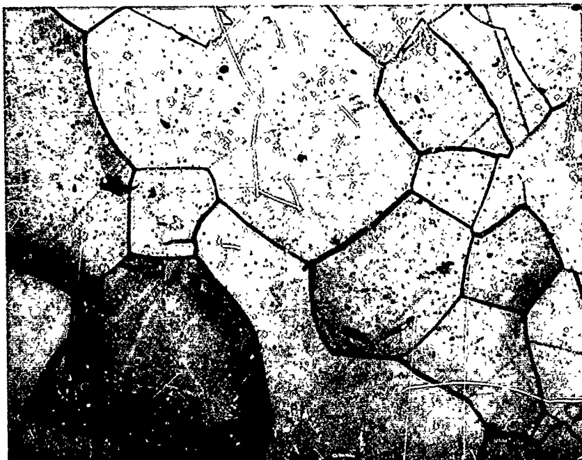
Figure 68. Iridium Sheet Annealed at 1650°C, (150X Magnification)
