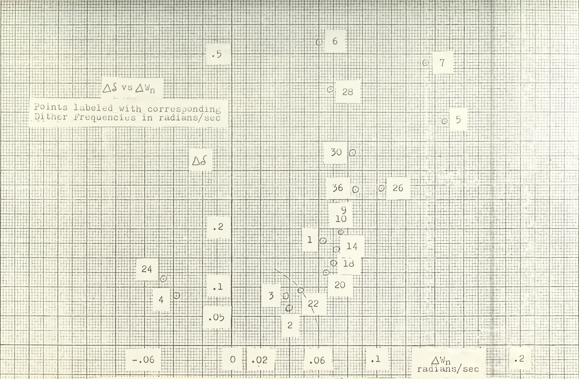
Figure 4.9. Variation in Damping Ratio vs Variation in Natural Frequency for Aerodynamic Condition 3.
