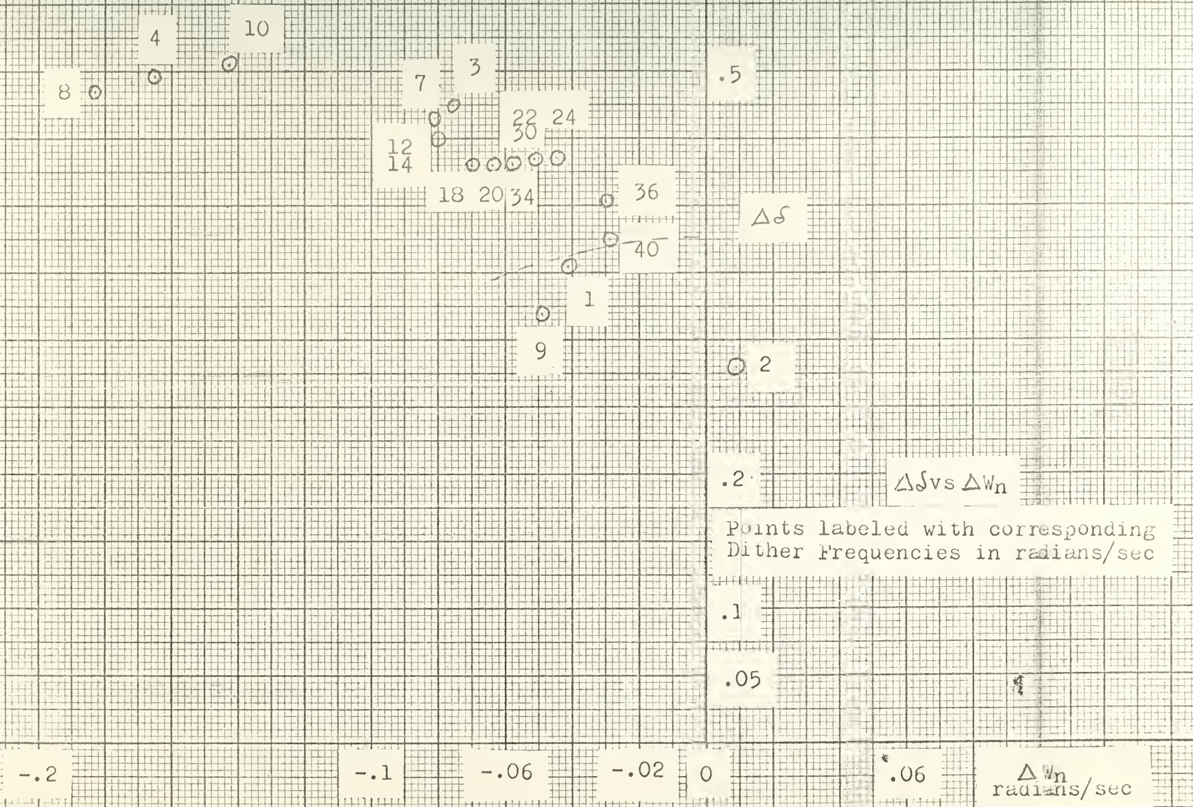
Figure 4.10. Variation in Damping Ratio vs Variation in Natural Frequency for Aerodynamic Condition 4.
