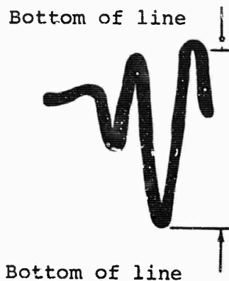
Detail Showing Allowance For Line Width
