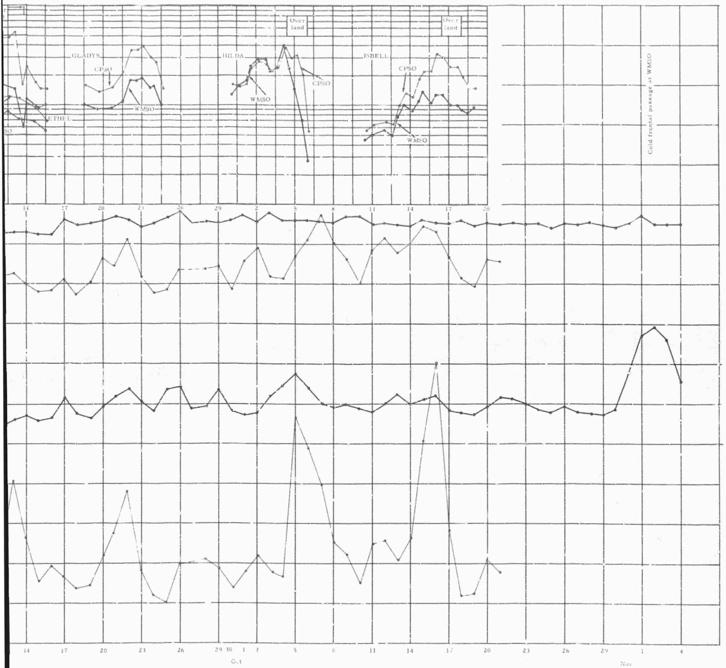
Figure 74. Correlation between microseismic background level and six hurricanes during the 1964 season at CPSO and WMSO
