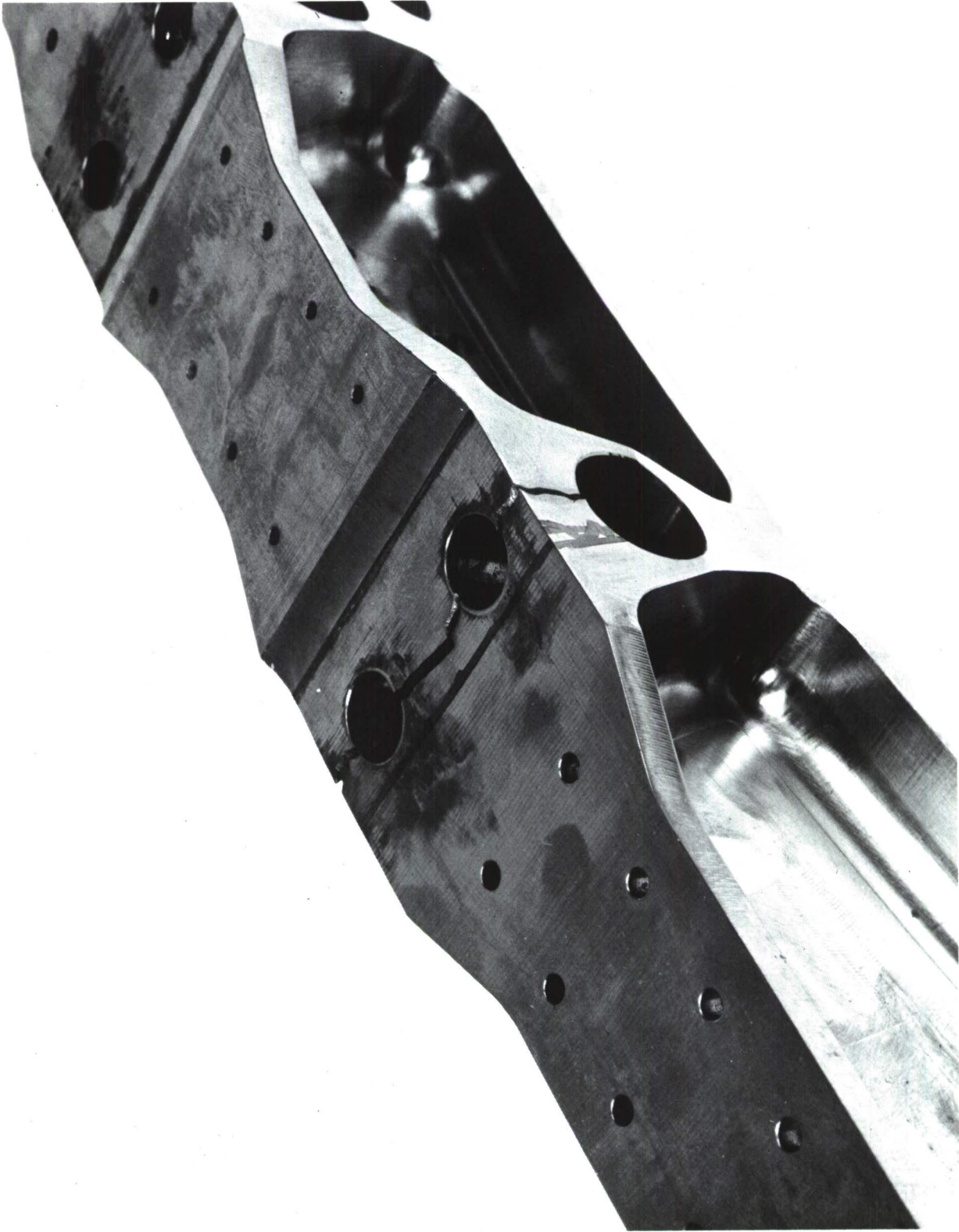
Figure 70. Fatigue Test Failure - IMI 679
