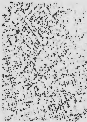
Figure 34. Zr-Hf-C: 59/31/10, Arc Melted X250 Primary Monocarbide Dendrites (Grey) in Metal Matrix (Light)
