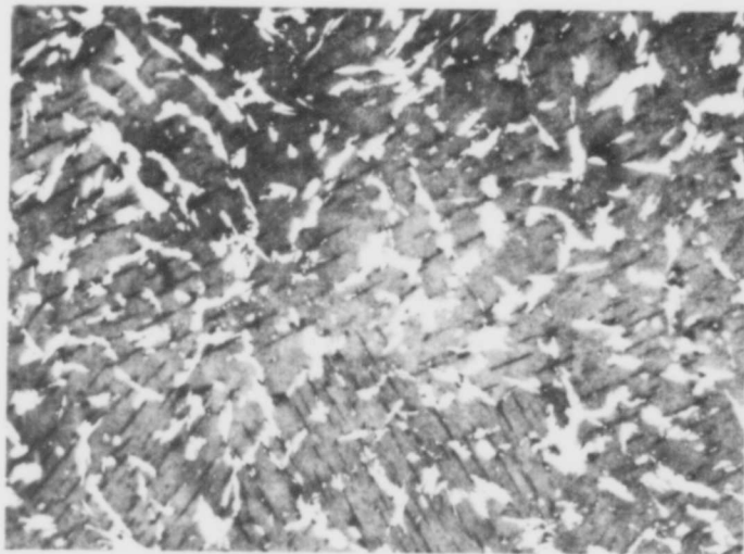
Figure 8. Hf-B (10 At% B), Quenched from 1900^{\circ}\text{C} .
