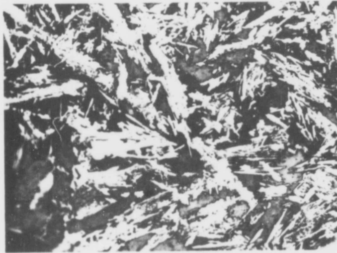
Figure 14. Hf-B (30 At% B), Cooled with 3°C per Second X1000 from 2130°C.
