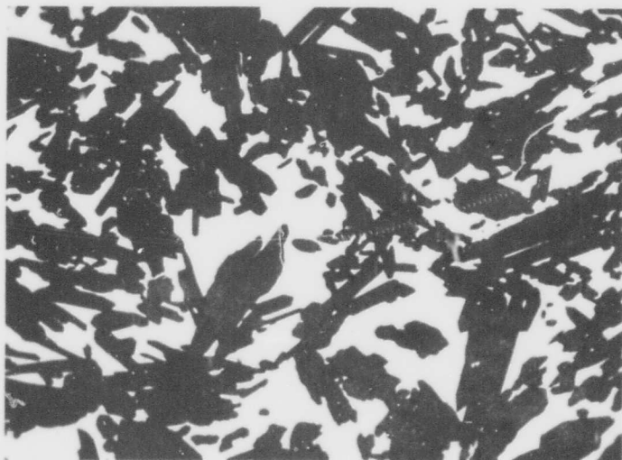
Figure 16. Hf-B (30 At% B), Alloy from Figure 14 Annealed for 225 hrs at 1650°C.
