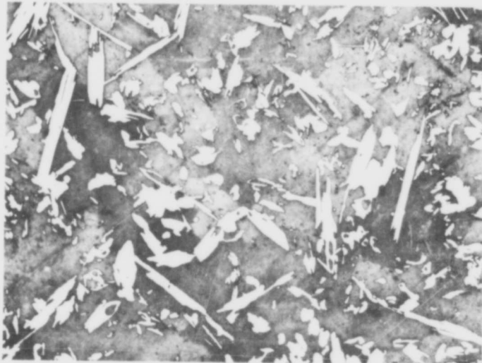
Figure 10. Hf-B (20 At% B), Quenched with \sim 8^\circ\text{C} per Second from 1900°C. X600
