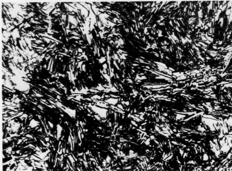
Figure 41. W-C (42 At% C), Quenched from 2730°C X400 \alpha -WC 1-x + WC Eutectic, with Traces of Primary Crystallized Tungsten Monocarbide (Light).
