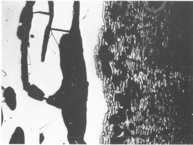
Figure 54. Molybdenum-Carbon Diffusion Couple, Interface B-C of the Sample in Figure 51.
