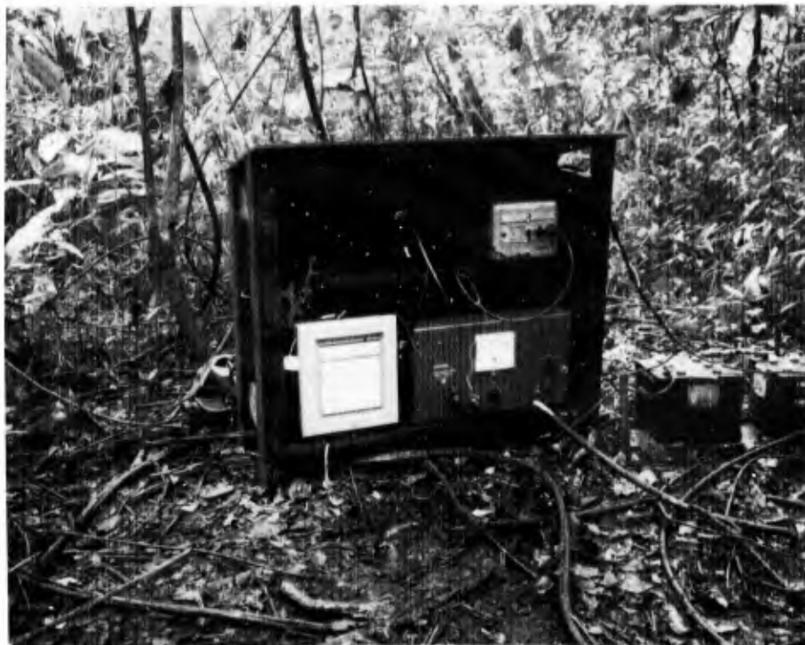
Figure 4. Recording apparatus for Illuminometer.
