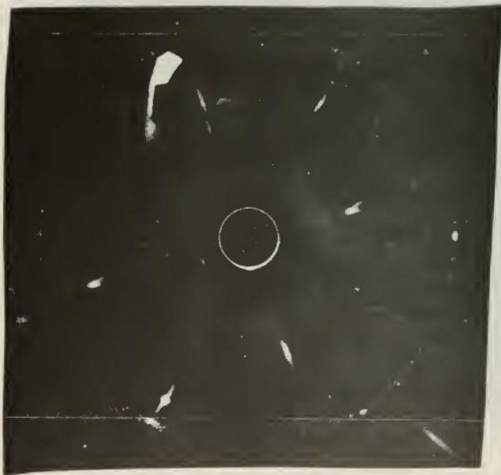
Figure 6. Laue transmission patterns of silver films having (100) orientation (upper) grown at 463^{\circ}\text{C} with mass 1.757 mg and (110) orientation (lower) grown at 437^{\circ}\text{C} with mass 1.757 mg.
