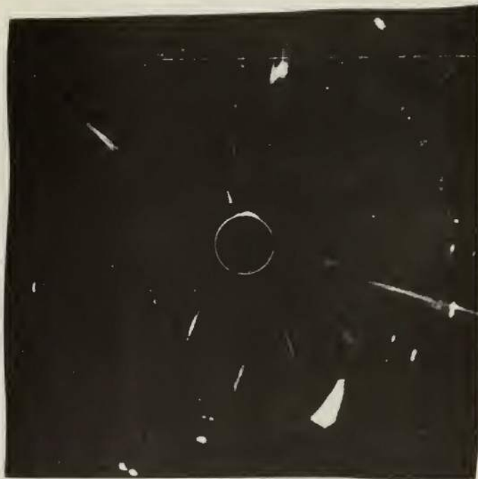
Figure 8. Laue transmission patterns of silver films having (100) orientation (upper) grown at 412^{\circ}\text{C} with mass 1.239 mg and (112) orientation (lower) grown at 433^{\circ}\text{C} with mass 1.251 mg.
