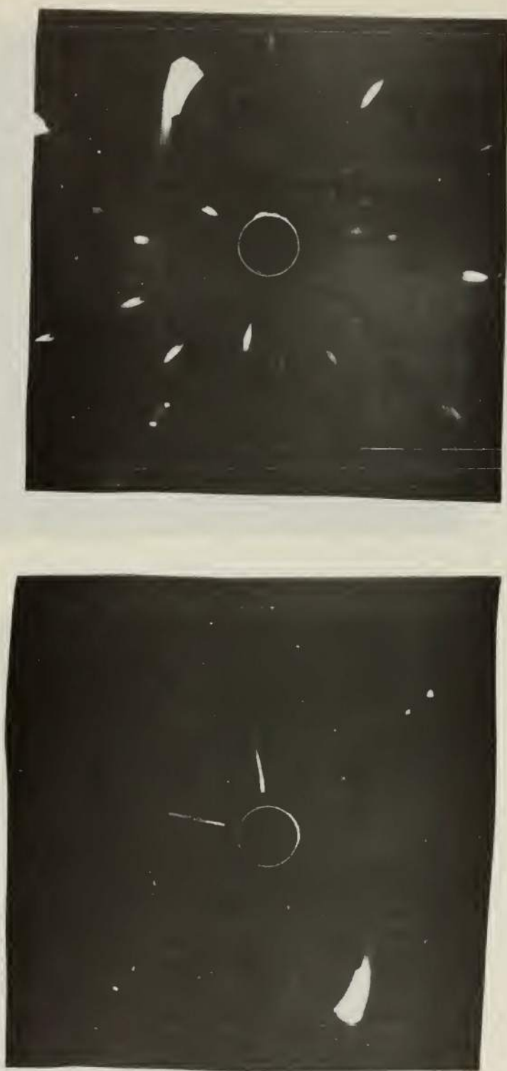
Figure 5. Laue transmission patterns of silver films having (112) orientation (upper) grown at 446°C with mass 1.929 mg and (110) orientation (lower) grown at 458°C with mass 1.922 mg.
