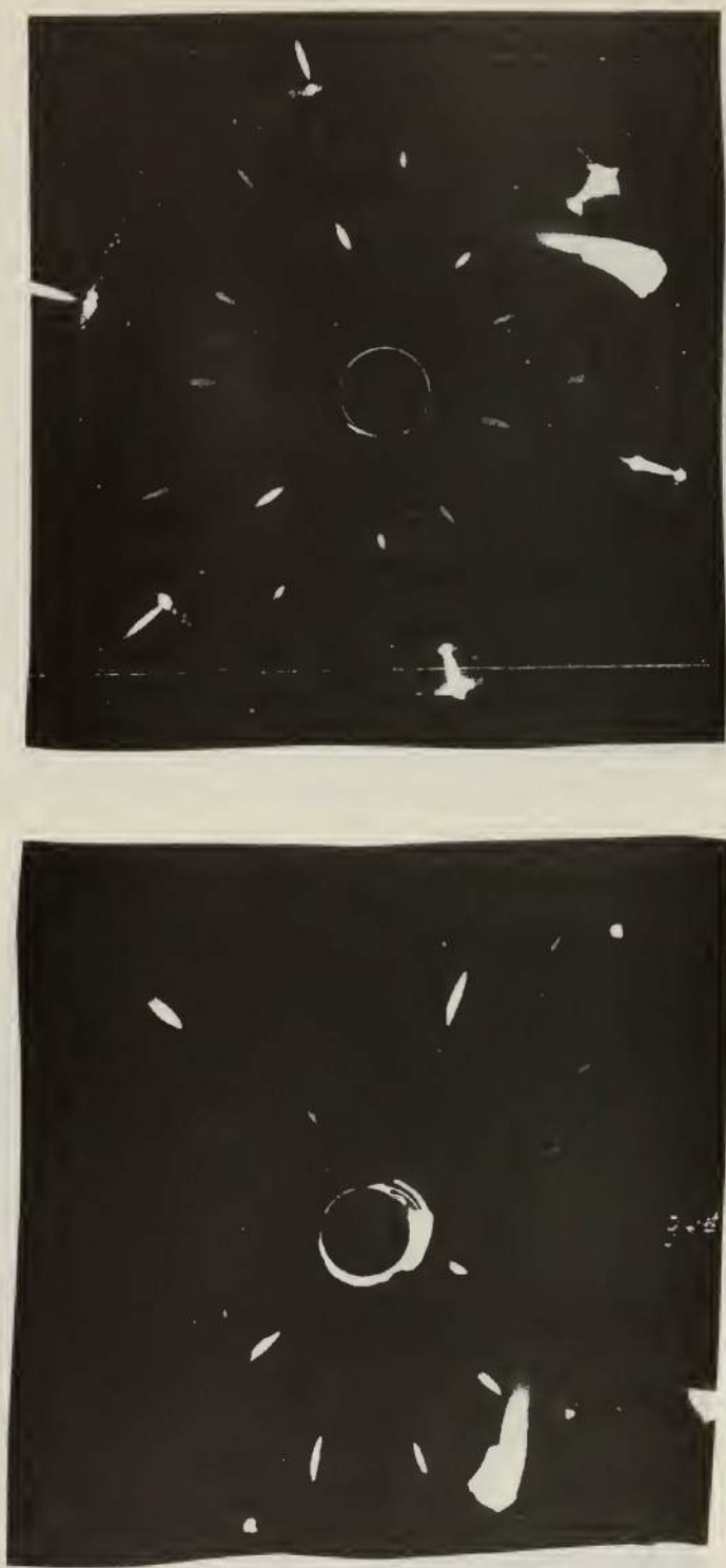
Figure 4. Laue transmission patterns of silver films having (111) orientation (upper) grown at 443^{\circ}\text{C} with mass 1.559 mg and (112) orientation (lower) grown at 430^{\circ}\text{C} with mass 1.537 mg.
