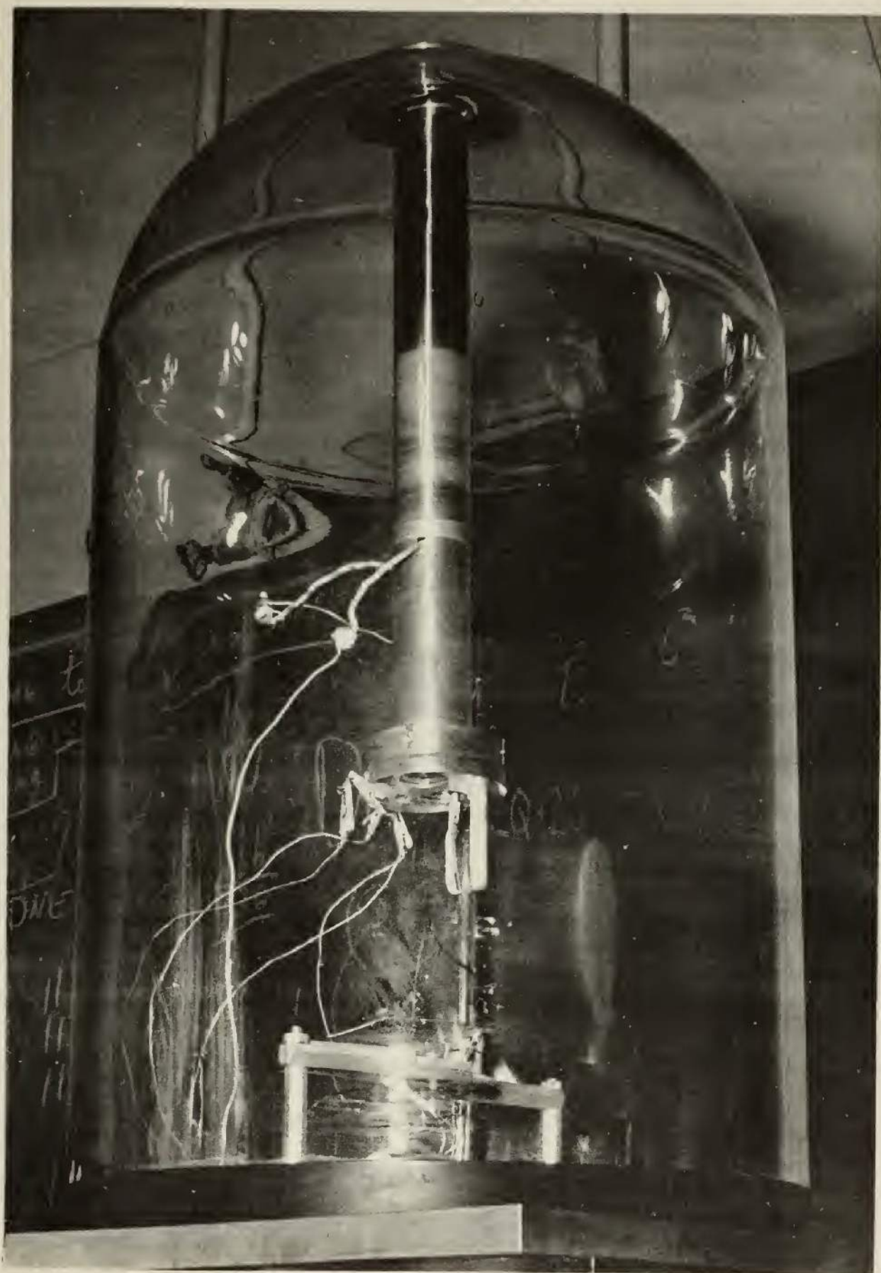
Figure 3. Complete evaporation assembly.
