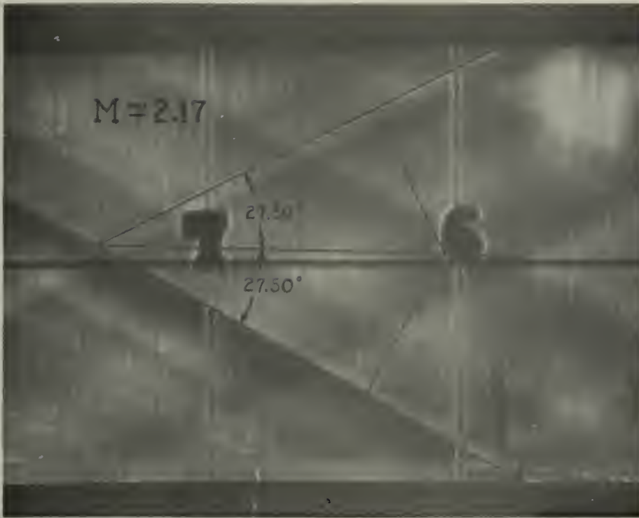
A. Vertical Knife. P_0 = 71.46 io. Hg. a. P_b = 30.92 io. Hg. a. T = 61.1^\circ F. Air Flow is Right to Left. Section is an Enlargement of Figure 13 A. Nozzle is Running Shock Free. Mach Number determined from Wavelets by Relationship \sin \alpha = \frac{1}{M} . At Corresponding Point Adiabatic Mach Number is 2.125.
