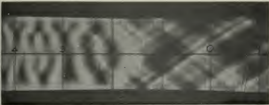
A. Vertical Knife. P_0 = 60.00 in. Hg. a., T_0 = 55.0^\circ F. Diffuser Height = 1.42 inches. Shock Pulled Back Through Diffuser Nozzle when P_0 was Decreased to 59.50 in. Hg. a.
