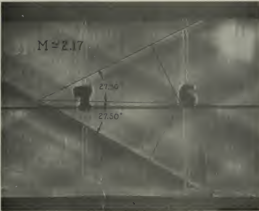
A. Vertical Knife. P_0 = 71.46 in. Hg. a., P_b = 30.92 in. Hg. a., T = 61.1^\circ F. Air Flow is Right to Left. Section is an Enlargement of Figure 13 A. Nozzle is Running Shock Free. Mach Number determined from Wevelets by Relationship \sin \alpha = \frac{1}{M} . At Corresponding Point Adiabatic Mach Number is 2.125.
