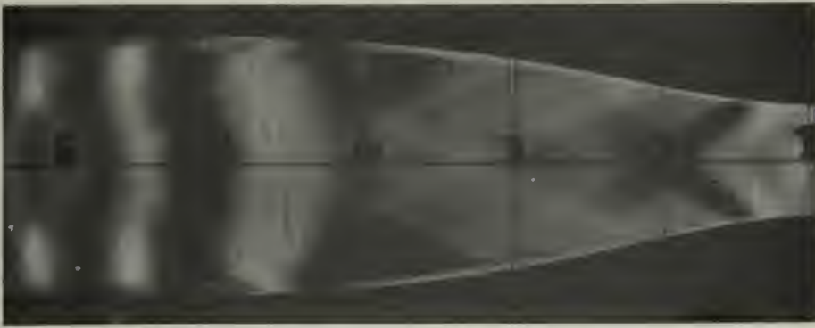
A. Vertical Knife. P_0 = 65.35 in. Hg. a., P_b = 30.65 in. Hg. a., T_n = 59.6^\circ F. Boundary Layer Visible on Nozzle Walls and Increasing in Thickness Downstream of Shock.
