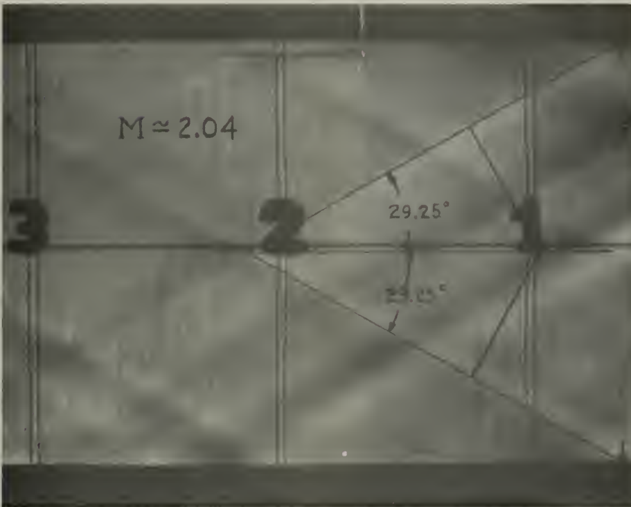
B. Vertical Knife. P_0 = 72.31 in. Hg. a., P_b = 30.92 in. Hg. a., T_0 = 59.23^\circ F. Air Flow is Right to Left. Section is an Enlargement of Figure 13B. At Corresponding Point Adiabatic Mach Number is 1.828.
