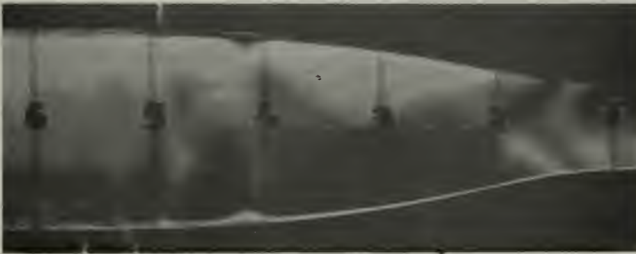
B. Horizontal Knife. P_0 = 64.41 in. Hg. a., P_b = 30.83 in. Hg. a., T_0 = 63.2^\circ F. Note Pull off of Boundary Layer at Shock and Asymmetrical Shading of Corres- ponding Parts on Opposite Sides of Tunnel Centerline. Shock is Moving Towards Nozzle Throat as P_n is Decreased from Figure 15 A.
