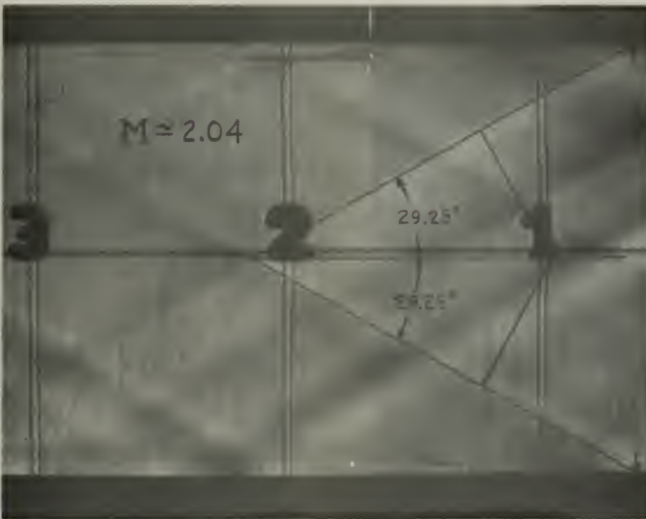
B. Vertical Knife. P_0 = 72.31 io. Hg. a., P_b = 30.92 io. Hg. a., T_0 = 59.23^\circ F. Air Flow is Right to Left. Section is an Enlargement of Figure 13B. At Corresponding Point Adiabatic Mach Number is 1.828.
