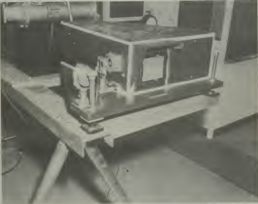
Figure 12. Schlieren System Light Source, Knife Edge, and Camera-Viewing Components.
