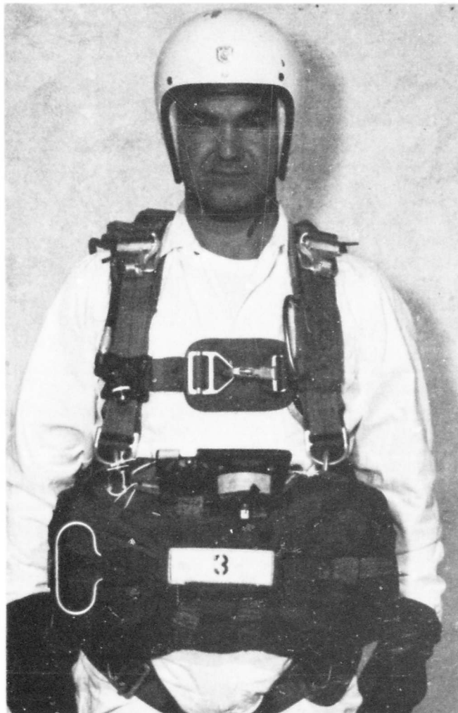
Figure 9 TEST PARACHUTIST PREPARED FOR LIVE JUMP WEARING PIONEER PARA-COMMANDER MARK I PARACHUTE ASSEMBLY WITH RESERVE
