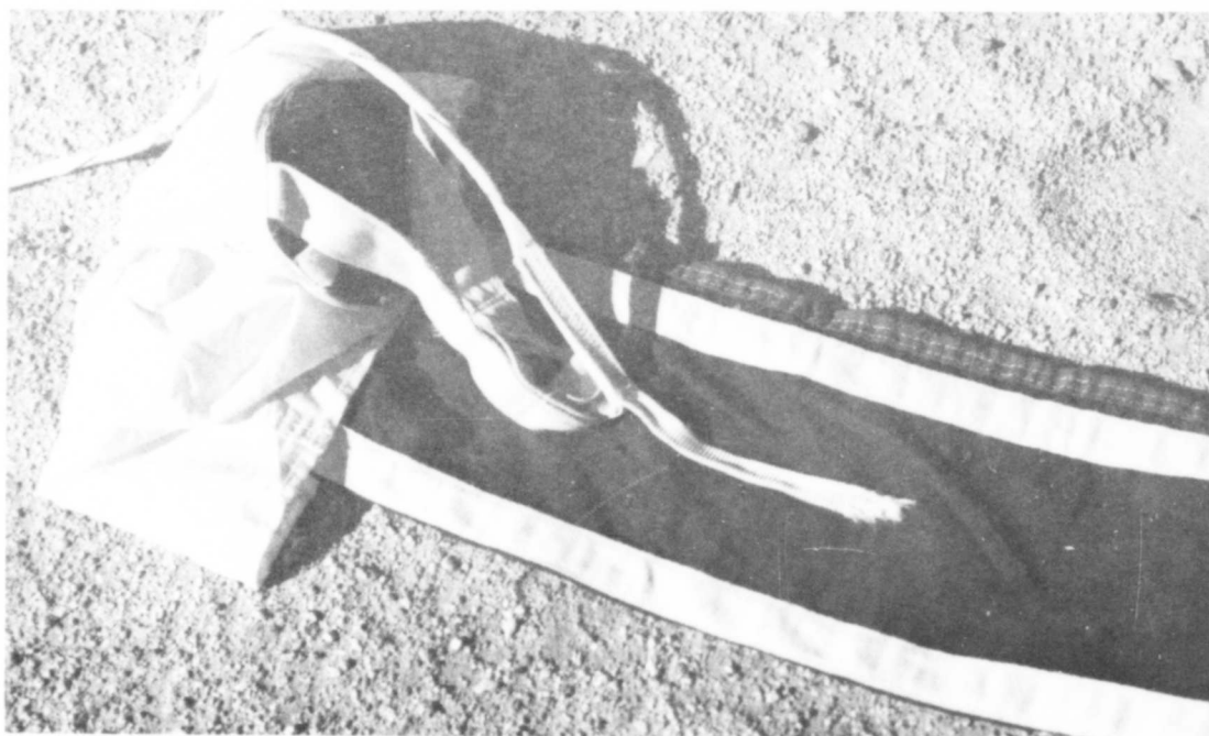
Figure 23 BROKEN 1500 lb (BREAK STRENGTH) TUBULAR NYLON WEBBING ON LAUNCH SLEEVE OF PIONEER PARA-COMMANDER MARK I PARACHUTE. FAILURE CAUSED LAUNCH SLEEVE TO SEPARATE FROM CANOPY DURING DROP TEST No. 1021 MADE AT 200 KCAS AND 1000 ft PRESSURE ALTITUDE.
