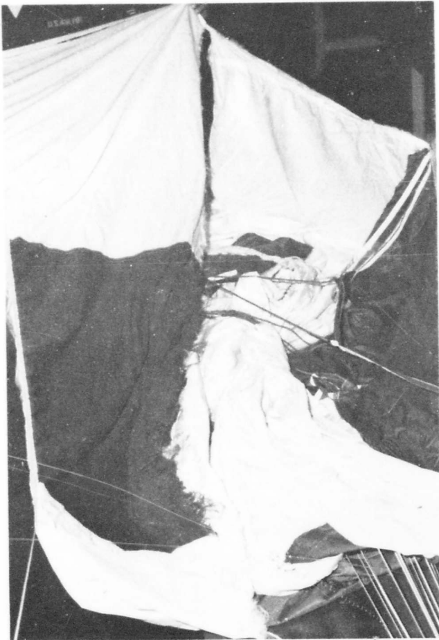
Figure 21 MAJOR DAMAGE TO STABILIZER PANEL OF PIONEER PARA-COMMANDER MARK I PARACHUTE CANOPY AFTER DROP TEST No. 1023 MADE AT 225 KCAS AND 1000 ft PRESSURE ALTITUDE.
