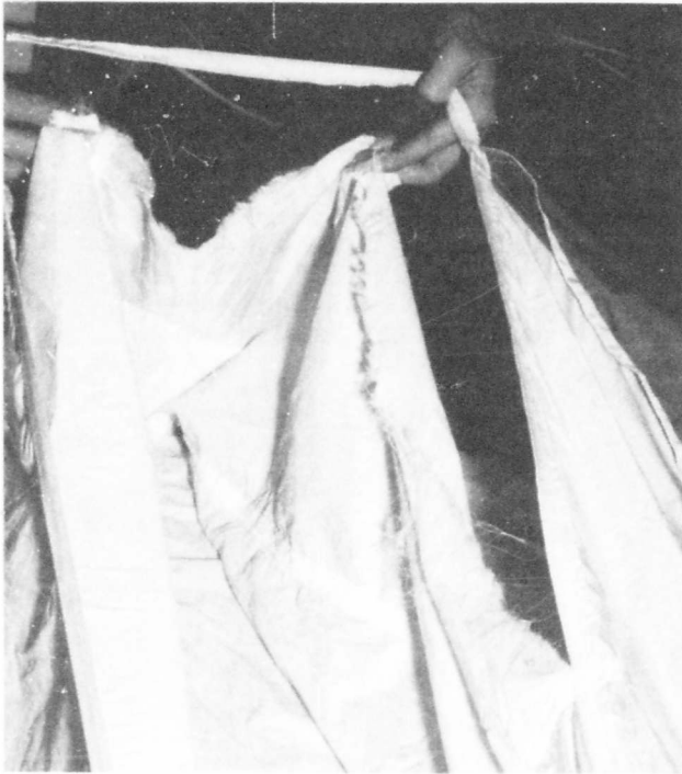
Figure 18 CANOPY OF PIONEER PARA-COMMANDER MARK I PARACHUTE SHOWING MAJOR DAMAGE AFTER DROP TEST No. 0516 MADE AT 170 KCAS AND 1000 ft PRESSURE ALTITUDE
