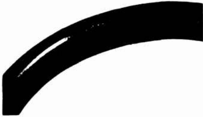
Figure 25. Source "B" - MIL-R-25897 O-Rings Tested Dynamically - Air-Aged
