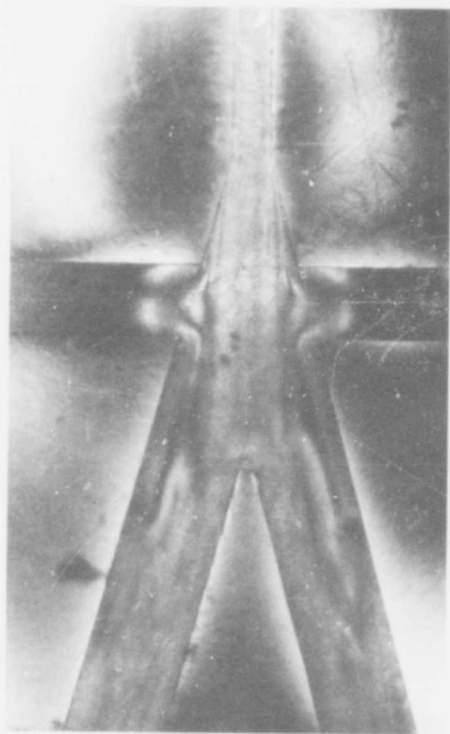
Figure 4. Flow Visualization in Bistable Test Element, Nozzle Pressure: 35\text{k Nt/m}^2
