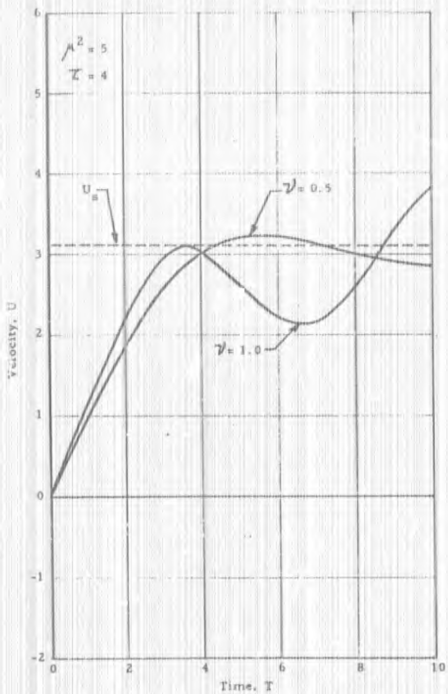
Fig. B-31. EFFECT OF ELASTIC BUFFER ON VELOCITY
