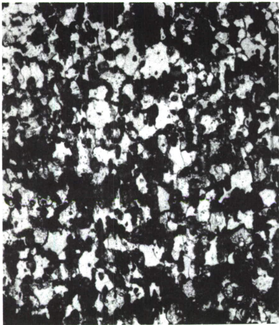
Figure 19A. Stress - 4000 psi Failure - 16.7 hours
