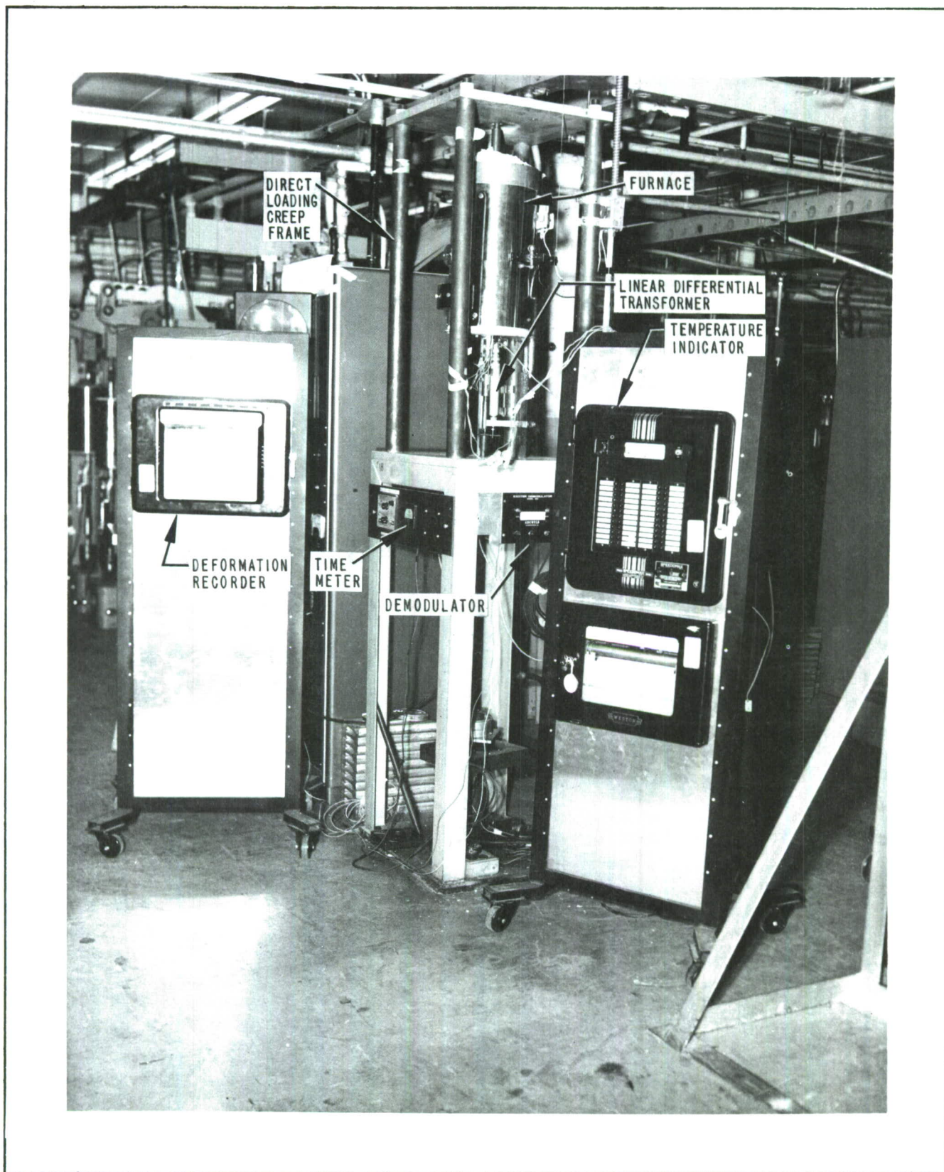
Figure 2. Test Apparatus Setup for Creep Rupture Tests
