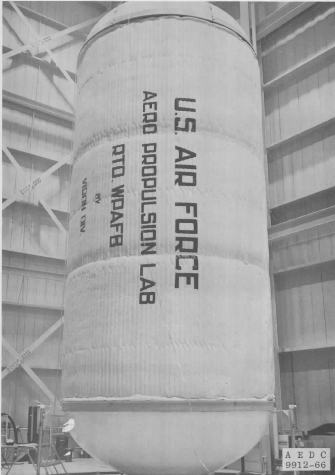
Fig. 6 Deployed Expandable Aerospace Shelter
