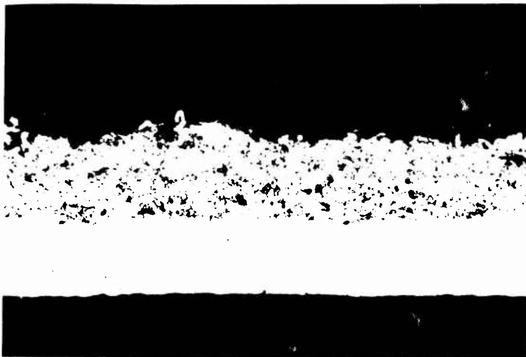
Figure 86. Flame-Spray-Metal on Bladder Shell
