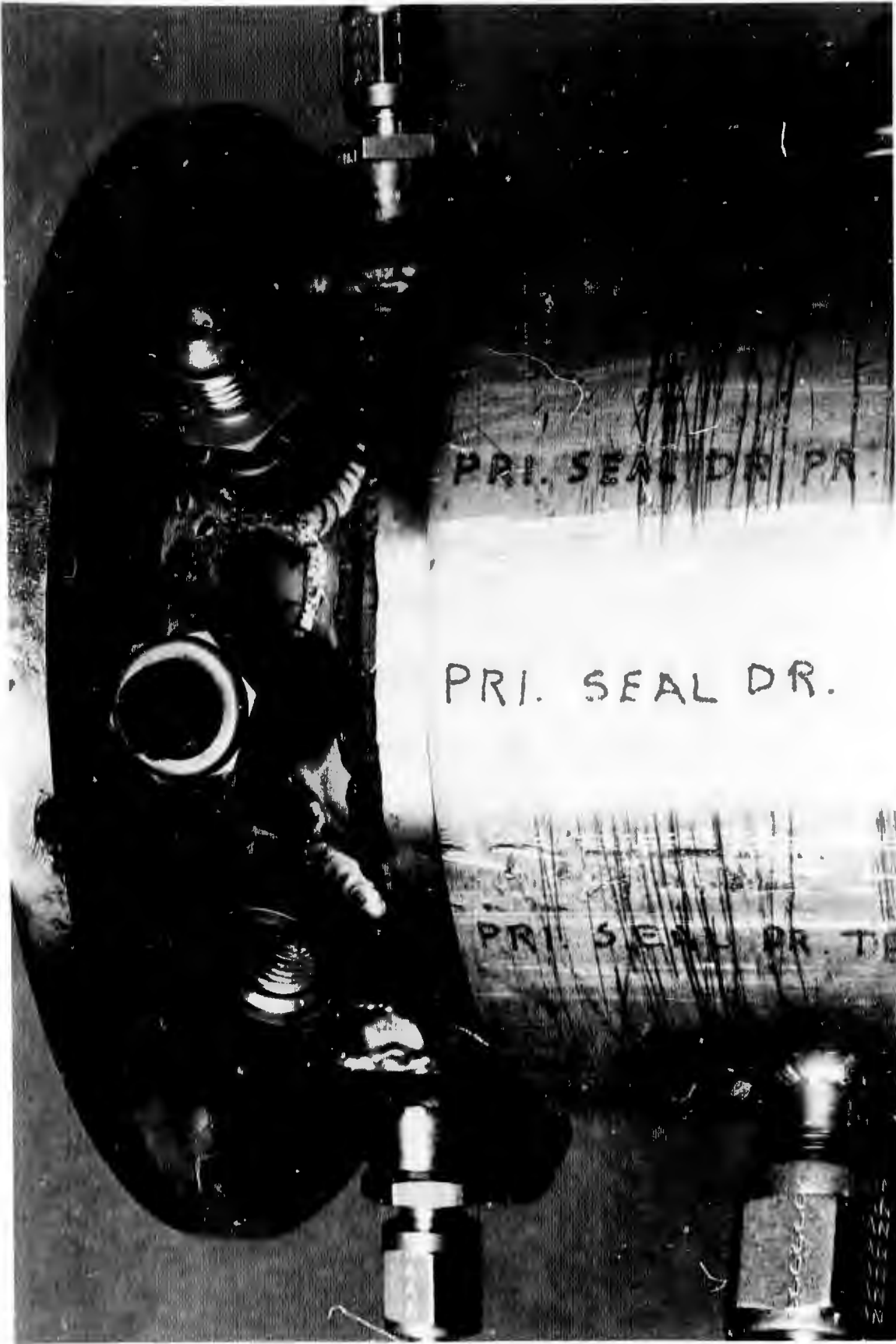
Figure 192. Main Tester Damage--View of Outer Housing Seal End (U)
