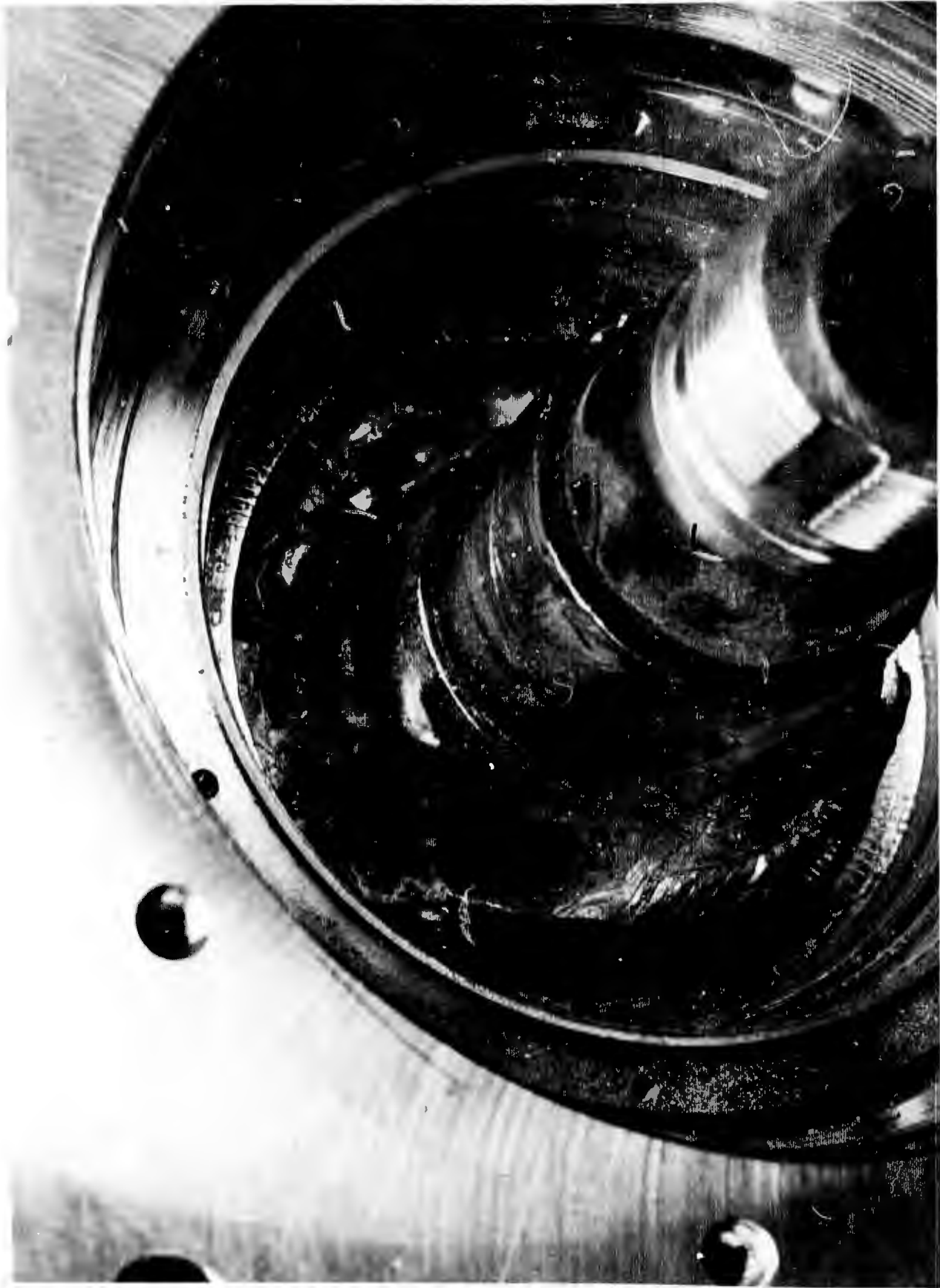
Figure 193. Main Tester Damage--View of Seal Cavity (U)
