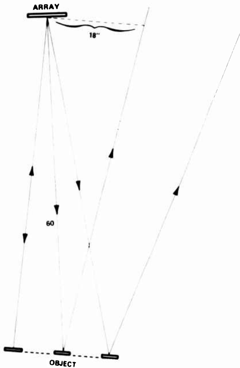
Figure 2-6 - Experimental arrangement to record hologram of 3-disc target
