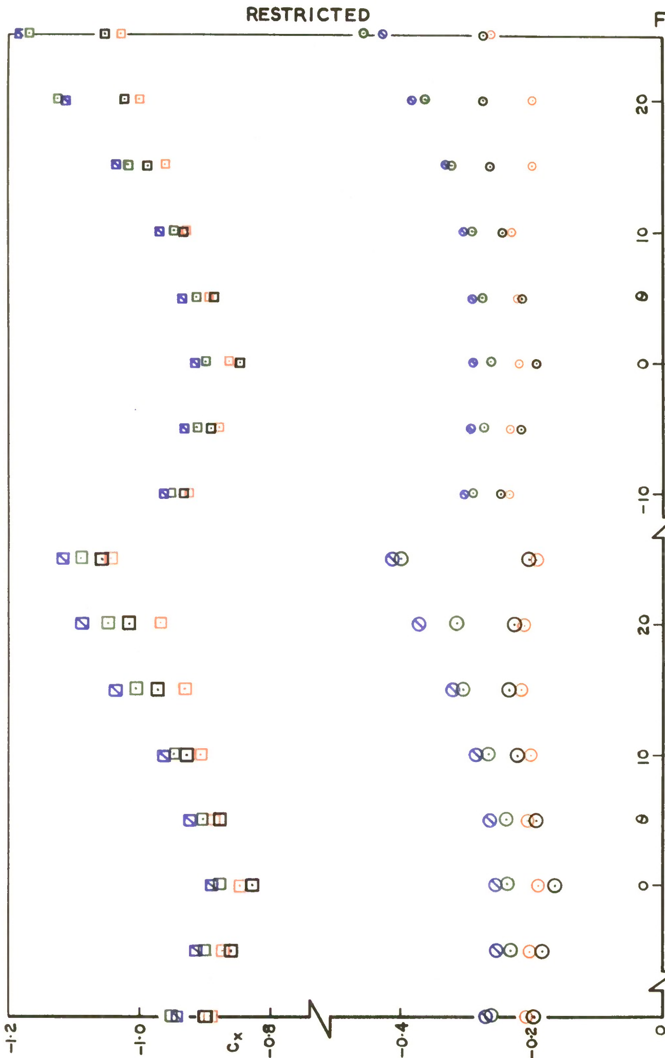
Fig. 11 Axial force on bomblets without fins and bomblets with uncanted fins
