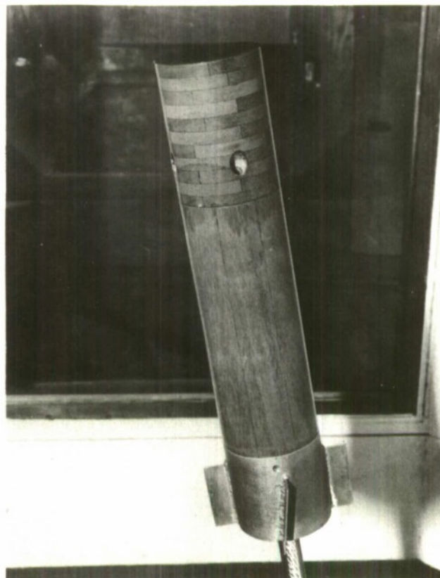
Fig.3. Bomblets mounted in the wind-tunnel. (Tail-retaining screws not fitted)
