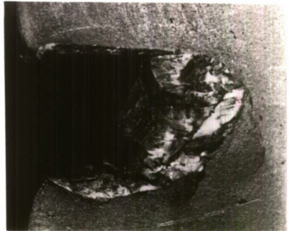
(b) PIECE OF ROD TRAPPED IN TARGET
