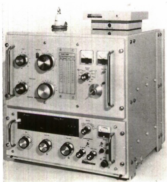
Fig. 1. 'Aries', 100W h.f. transmitter type H1030
