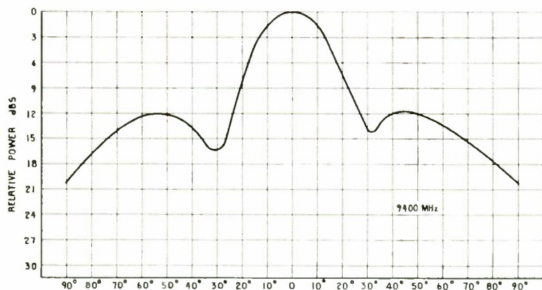
FIG. 9. 2 Stack Curved Array— —Vertical Radiation Pattern.
