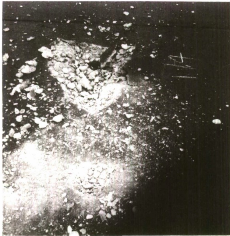
FIG. 7 (a) WEST FREUGH CRATER PRODUCED BY 5 in DIAMETER SHAPED CHARGE
