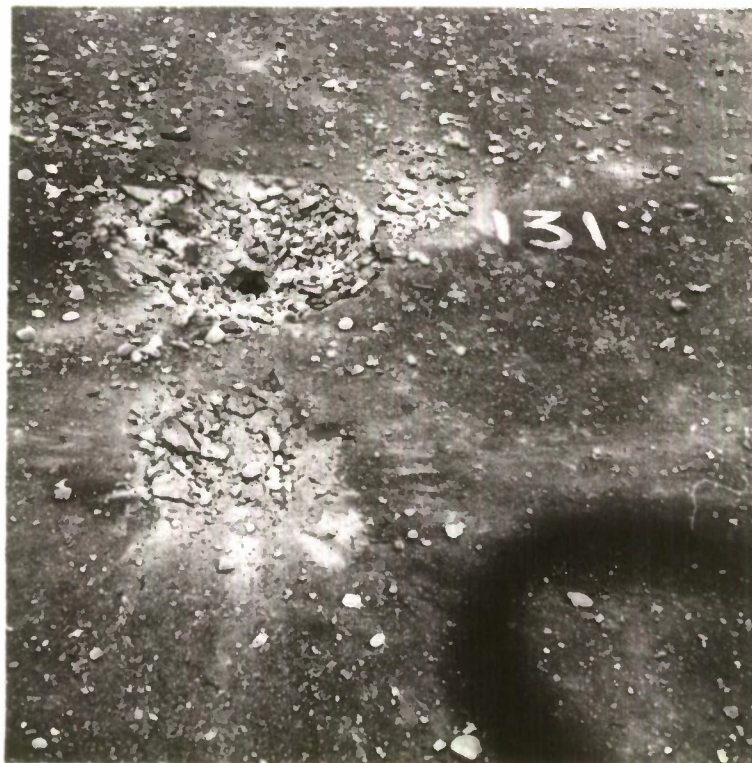
FIG. 7 (b) WEST FREUGH CRATER PRODUCED BY 7 in DIAMETER SHAPED CHARGE
