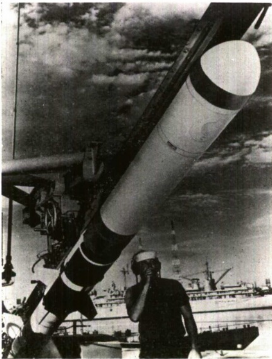
FIG. 46. "ASROC" booster carrying lightweight torpedo (Mk. 44 or Mk. 46).
