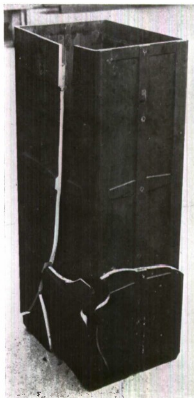
FIG. 1. Old Lorival container following shock. Showing bearers for lid.
