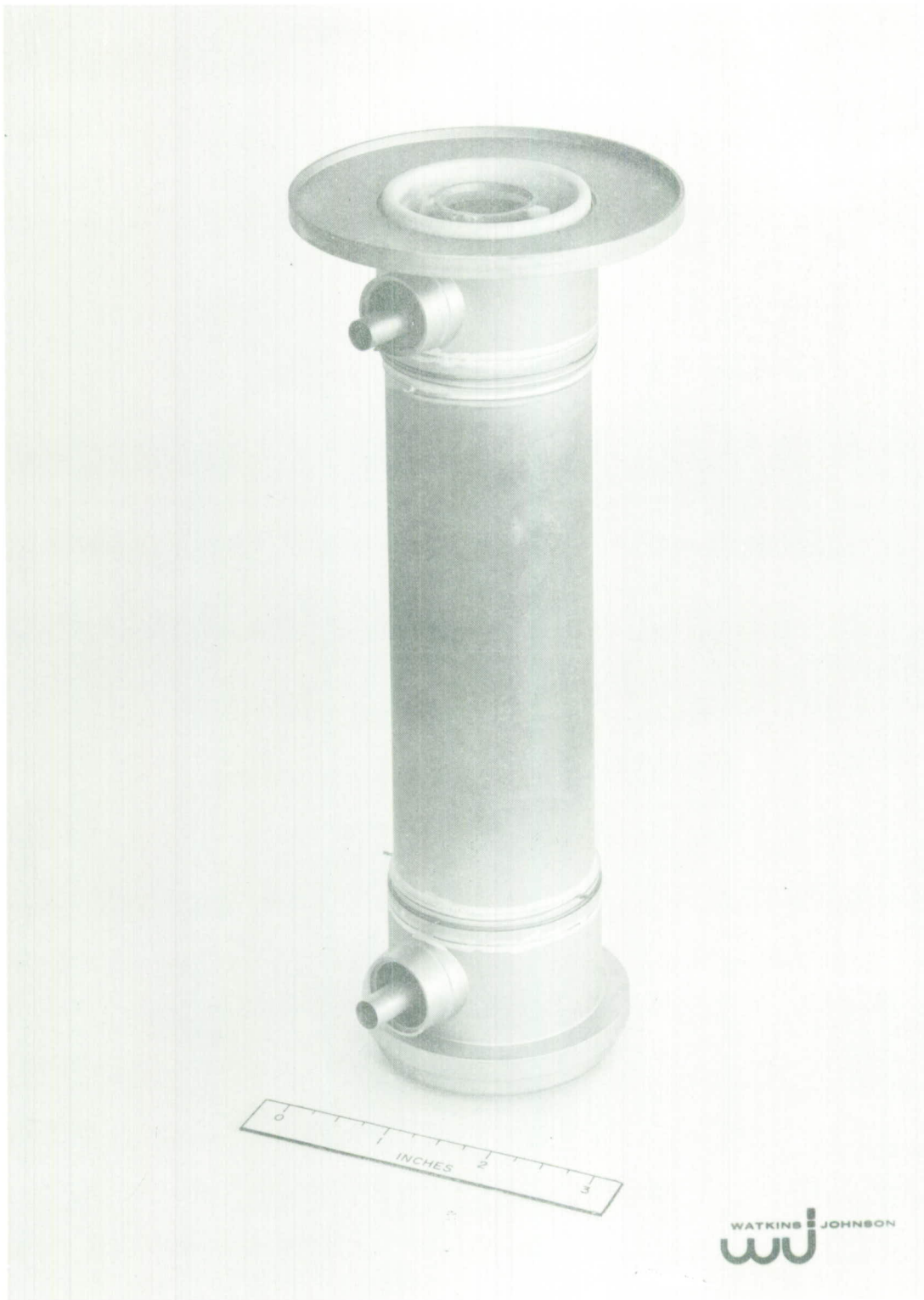
Fig. 24 - The photograph shows the ceramic barrel and circuit assembly as used in the first grounded cathode tube.
