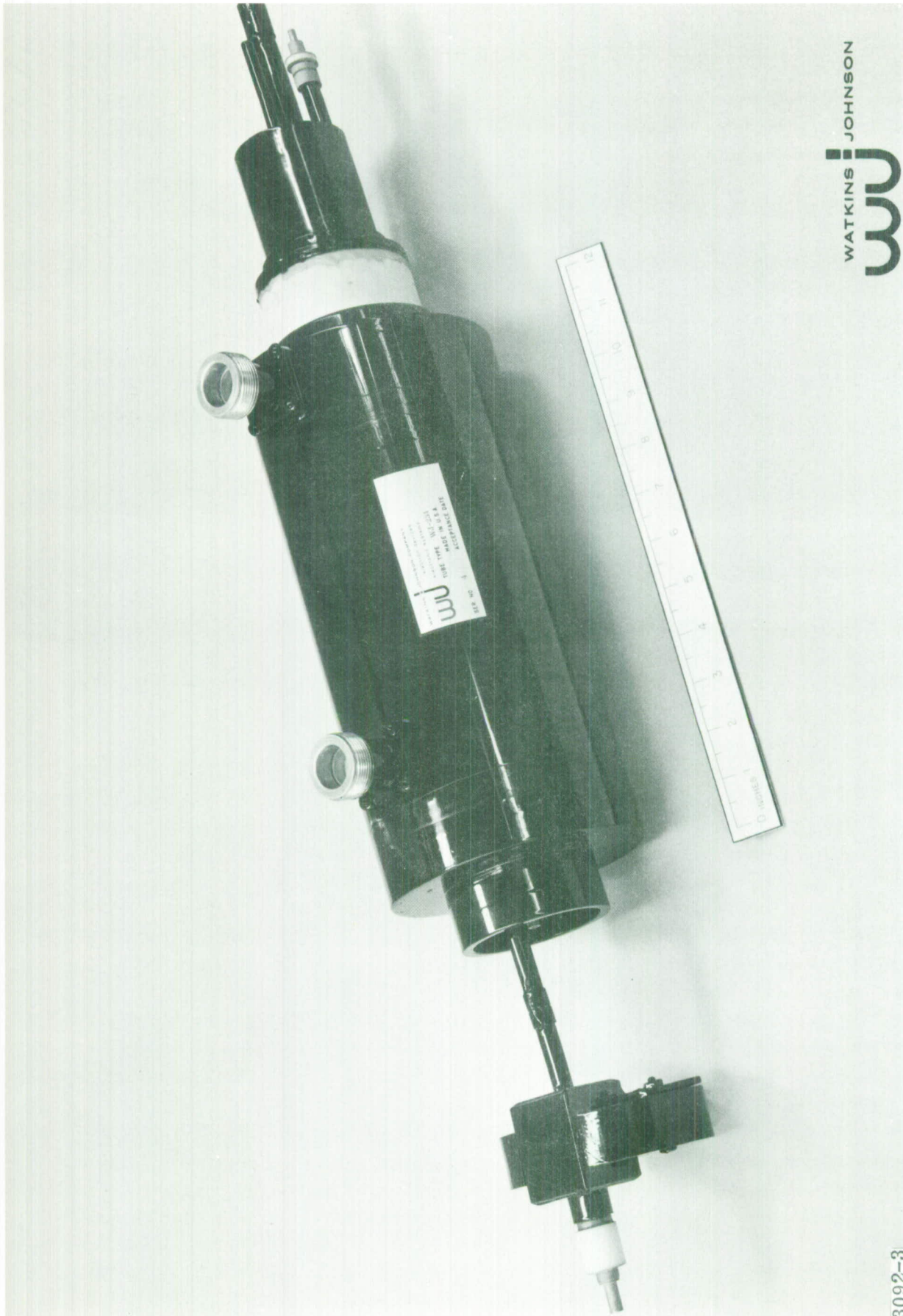
Fig. 41 - Photograph of the ceramic grounded cathode tube. The tube is focused by means of a single reversal ceramic magnet stack. Figs. 42 and 43 are plots of data measured on the ceramic barrel tube. Table III lists the operating parameter of the tube.
