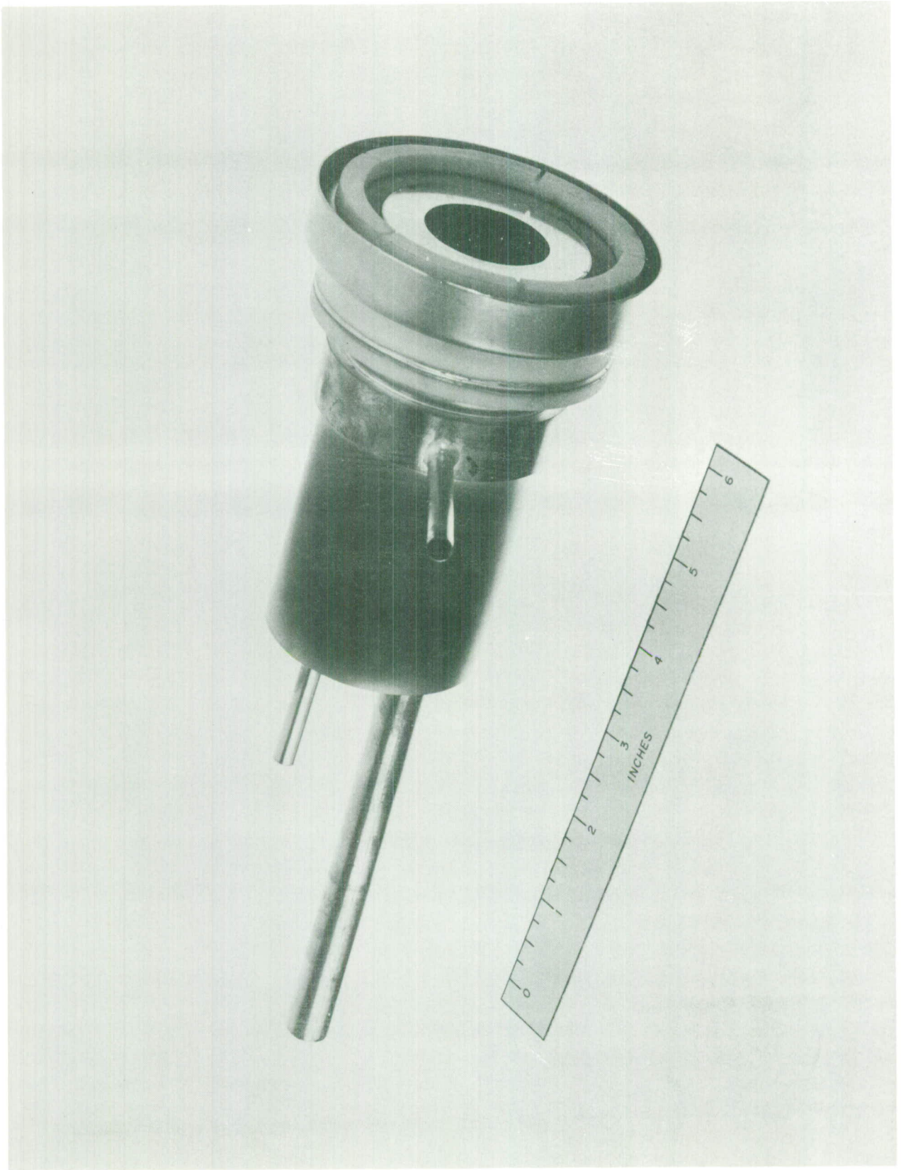
Fig. 17 - A collector assembly for the L-band amplifier.
