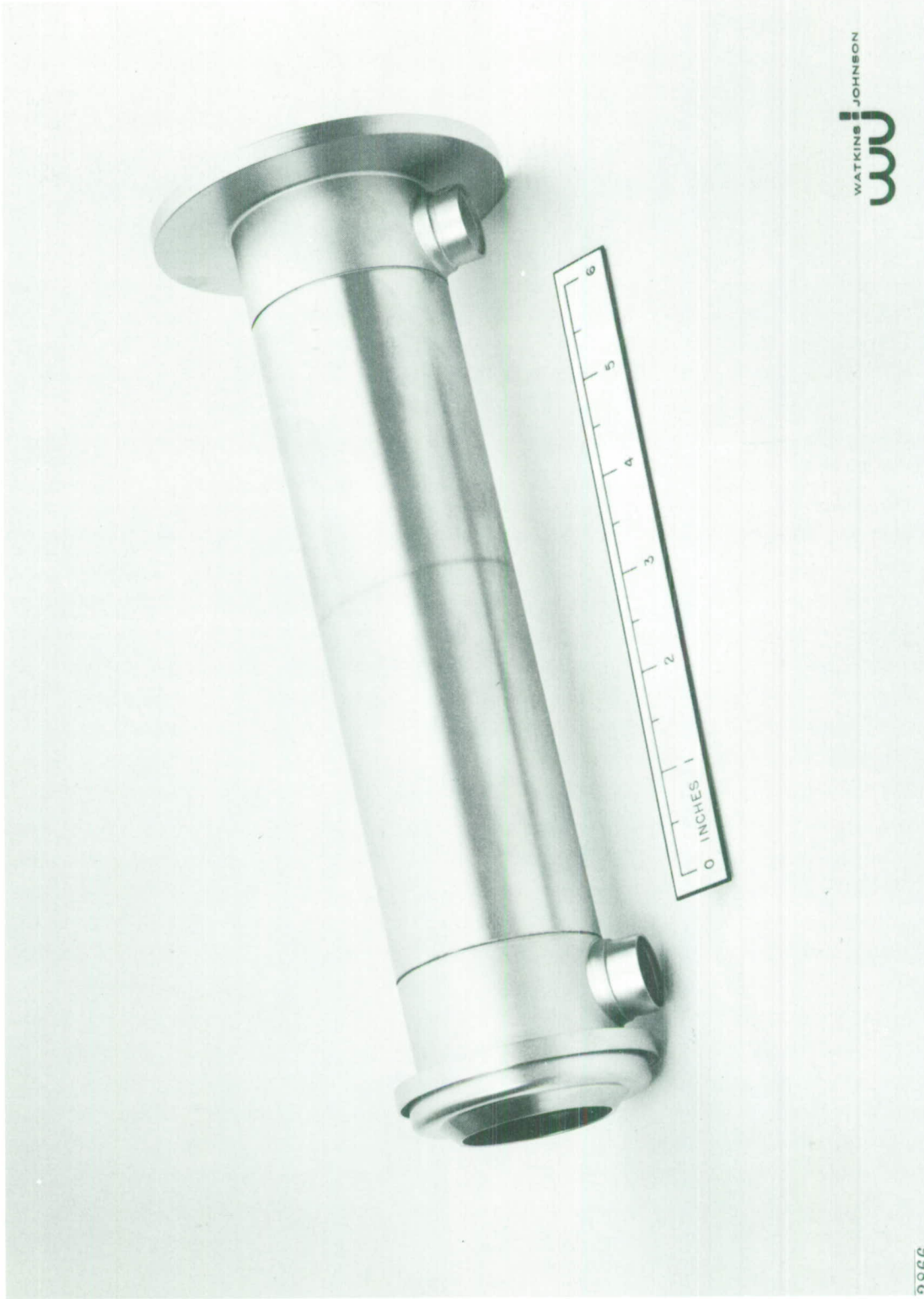
Fig. 38 - Metal barrel assembly for the grounded cathode tube.
