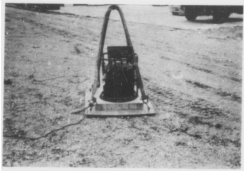
Figure 1 - Sterilizer Rigged to Platform Prior to Static Drop
