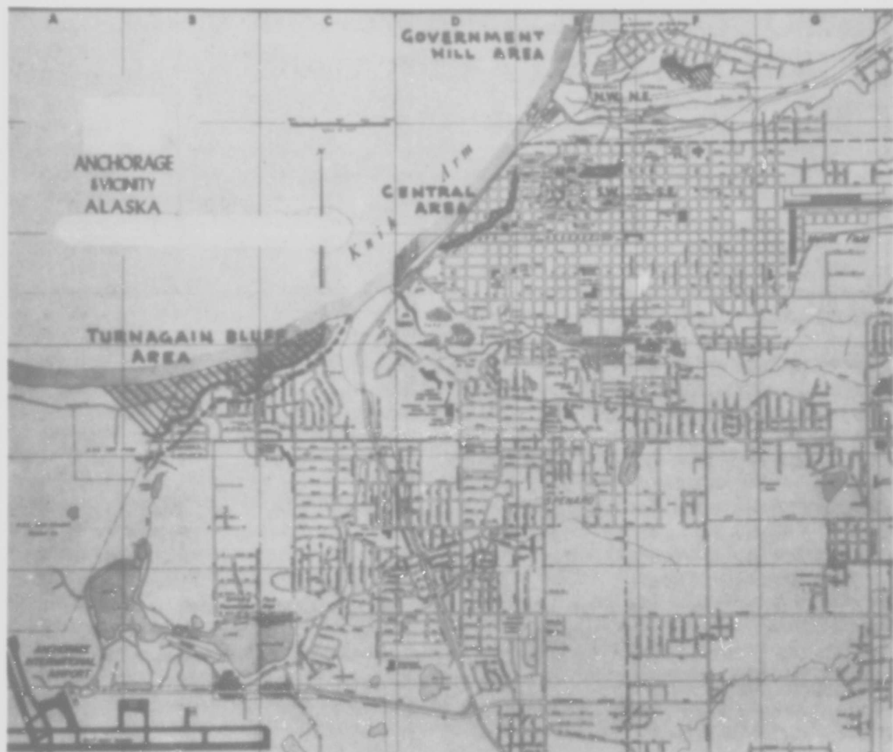
Figure 2.--Anchorage. The large cross-hatched area on the left is the Turnagain bluff housing area where damage to houses was caused by major earth slides.
