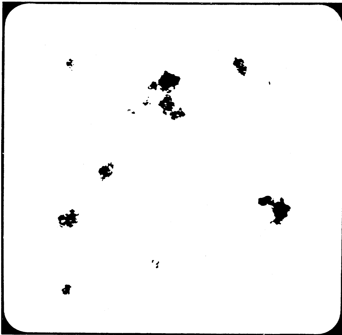
Fig. 8 J. T. Baker Thermistor Grade Cobalt Oxide Powder 8.5 m 2 /gram, Unsintered 15,000X
