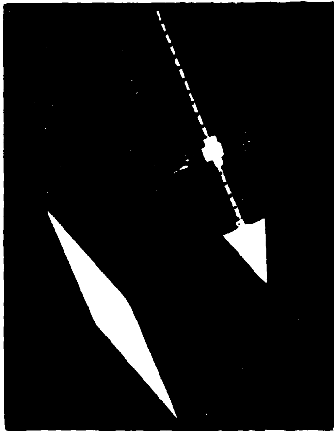
FIG 14-5. CLOSE-UP OF KNIFE EDGE ASSEMBLY AND PRISM FOR SCHLIEREN SYSTEM.
