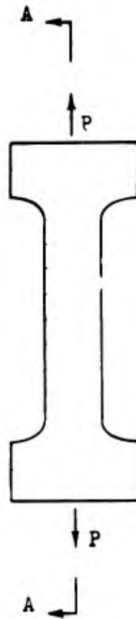
Fig. 1b A Spiralloxy specimen with filaments normal to the applied force
