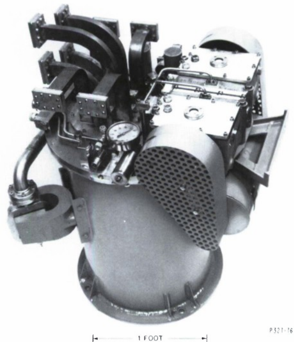
Fig. 41. Air Products closed-cycle refrigerator with four 2-stage amplifiers to be used in later tests.
