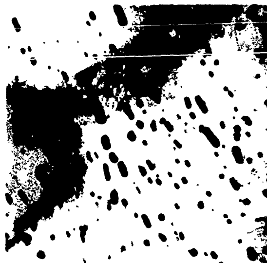
(b) Al-4.3 percent Cu aged at 0°C after solution treatment Precipitate density \sim 5.0 \times 10^9 \text{ cm}^{-2}
