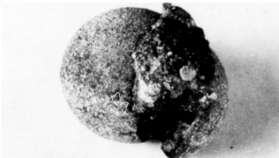
Figure 74. Appearance of JTA Sample After Being Tested for 11 Minutes at 1900°C
