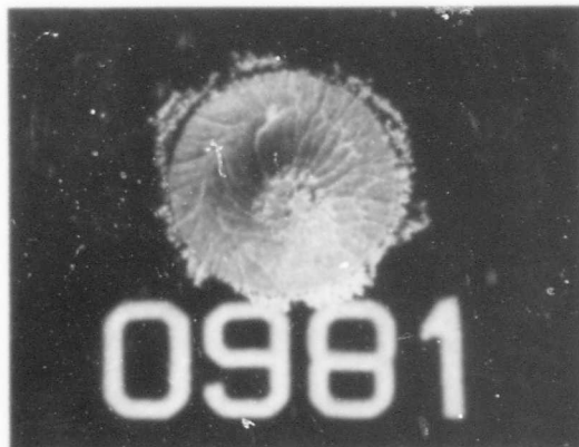
Figure 102. Front View of JT-0981 After Sonic Air Plasma Exposure at a Front Surface Temperature of 2300^{\circ}\text{C} , Test Duration, 200 Sec.
