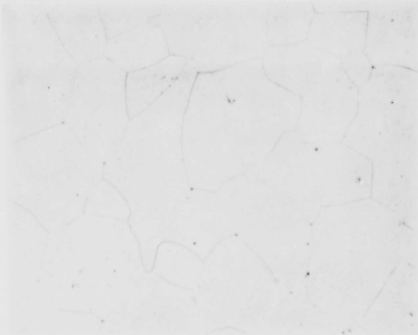
Figure 3- Grain structure of 21 a/o Cb standard after 12 hour homogenization anneal at 1300°C. Etchant 2 parts H_2SO_4 , 2 parts HNO_3 , 1 part 52% HF. 250X.
