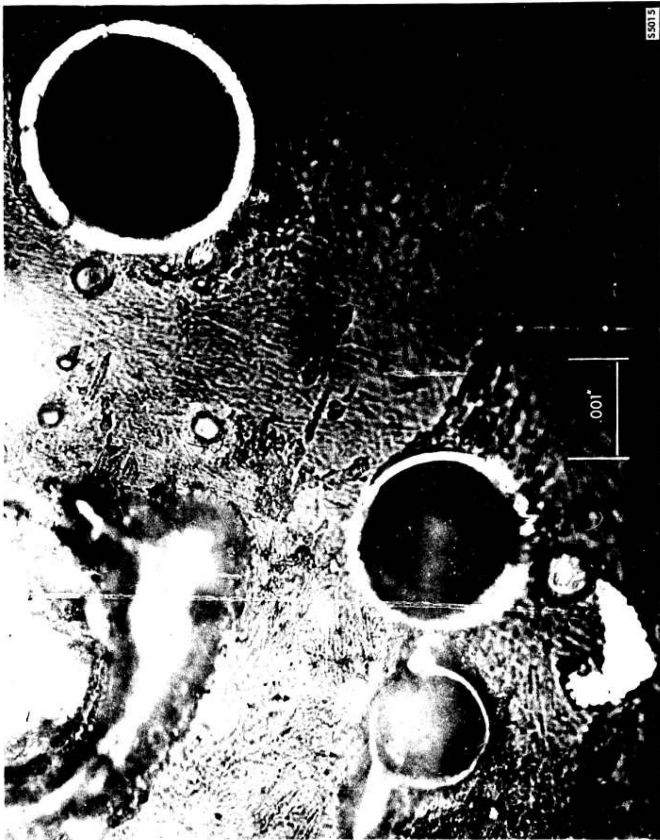
FIGURE 1. CROSS SECTION OF ALUMINUM ALLOY COMBUSTION PRODUCTS SHOWING SPHERICAL OXIDE SHELLS
