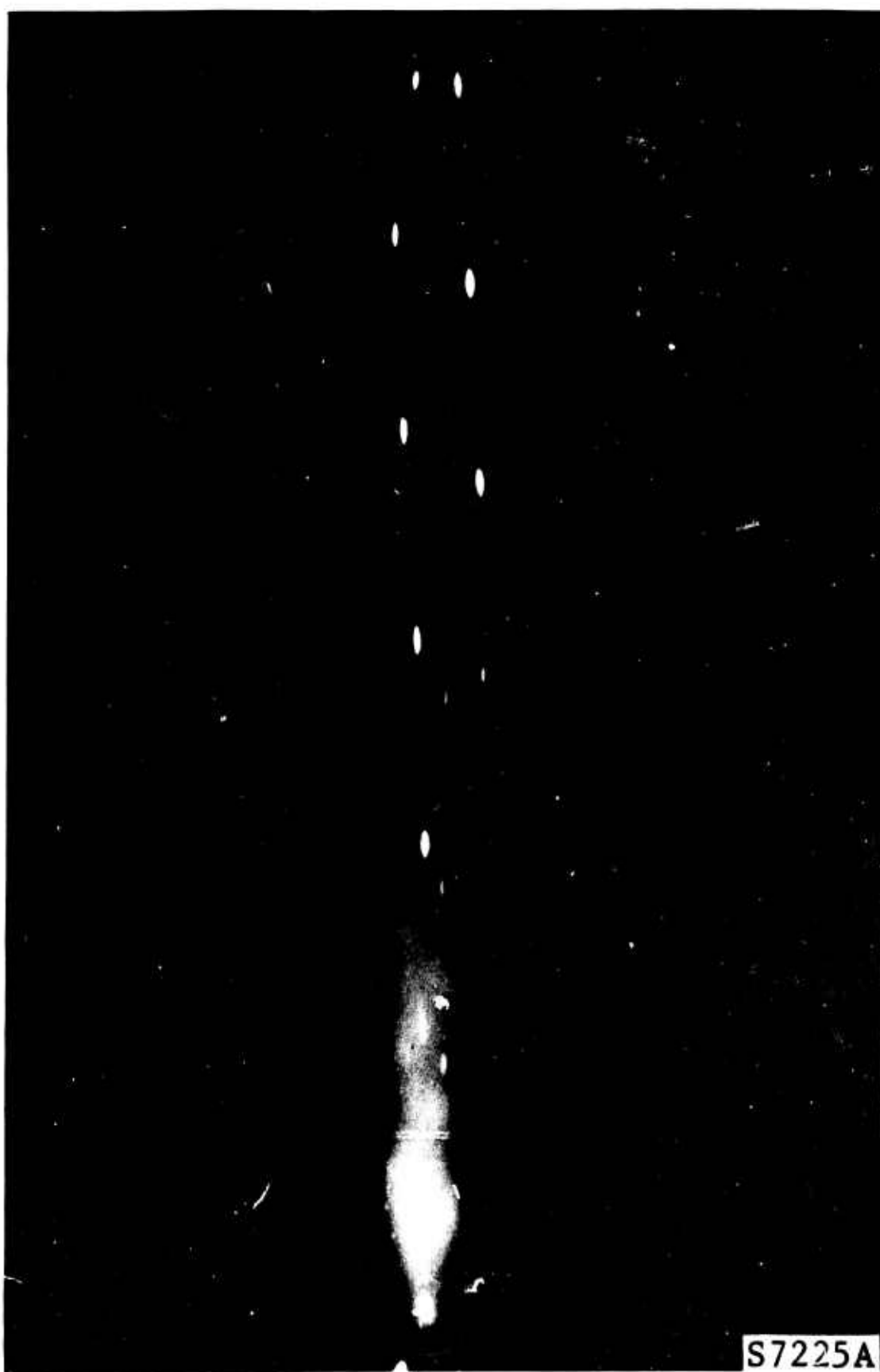
FIGURE 2. MIXTURE OF -115 +150 MESH ALUMINUM AND MAGNESIUM PARTICLES BURNING IN AN OXYGEN-NATURAL GAS FLAME; PHOTOGRAPHED THROUGH A 160-INTERRUPTIONS-PER-SECOND LIGHT CHOPPER
