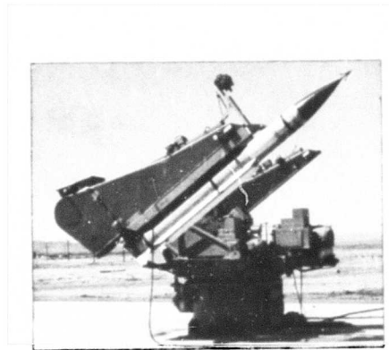
FIG. 19. Tartar Missile Mounted on Guided Missile Launcher Type X-7.
