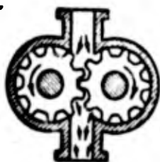
Figure 187. Diagram of the spur-gear pump.
