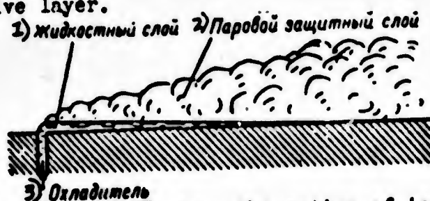
Figure 110. Diagram to show the action of internal cooling.
