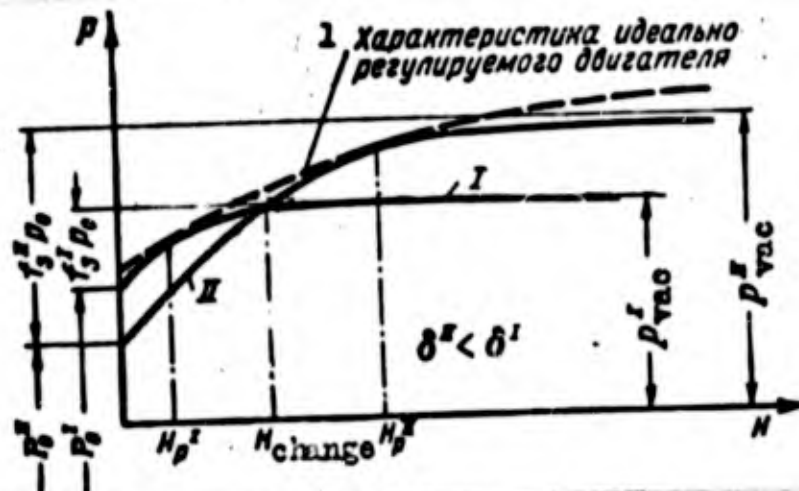
Figure 74. The altitude characteristics of two engines with different values of the nozzle area ratio.
