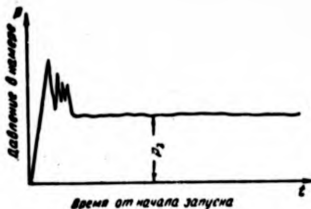
Figure 149. Change of pressure in starting a liquid-fuel rocket engine.
