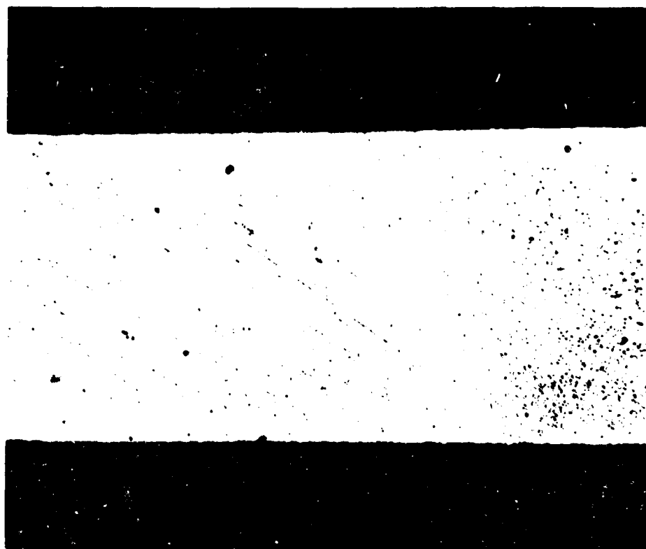
Figure 21 - Photomicrograph of seal sample T-5A, transverse section, after 1000 hours at 900°C in 1 Torr of cesium vapor, 250 X
