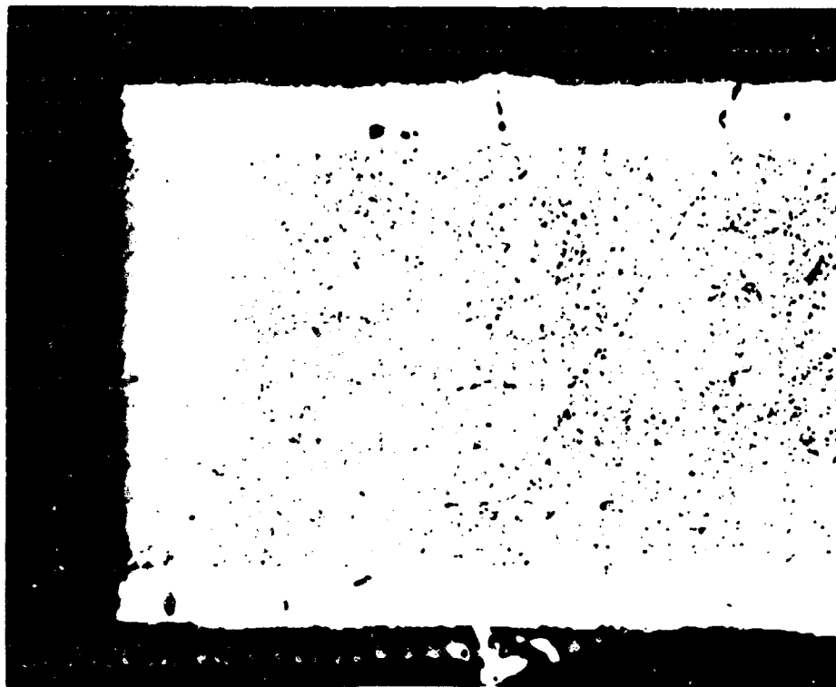
Figure 25 - Photomicrograph of seal sample T-5A, longitudinal section, after 1000 hours at 900°C in 1 Torr of cesium vapor, 250 X
