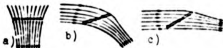
Fig. 9.1. Airflow conditions of rotor. a) axial airflow; b) transitional airflow (small values of \mu ); c) oblique airflow (large values of \mu ).
