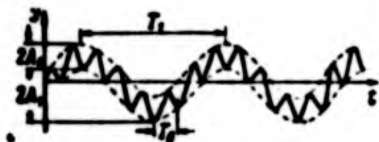
Fig. 10.40. Breakdown of a curve which consists of two sinusoids with frequency ratio 6 : 1.
