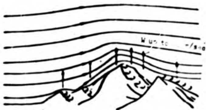
Fig. 1.14. Influence of relief of surface of earth on vertical air flows.
