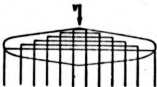
Fig. 6.12. Diagram of vortices in the air flow around a wing.
