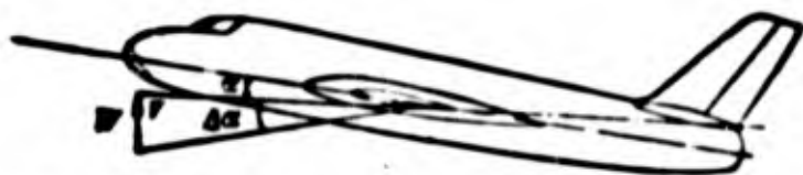
Fig. 1.17. Diagram of influence of vertical gust on aircraft.
