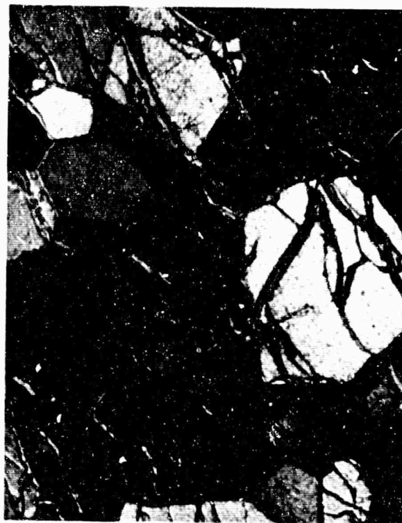
Figure 17. Thin Section of North Carolina Olivine Showing Serpentine Adjacent to and Along Cracks in the Olivine Grains. Largest grains are 2 mm across
