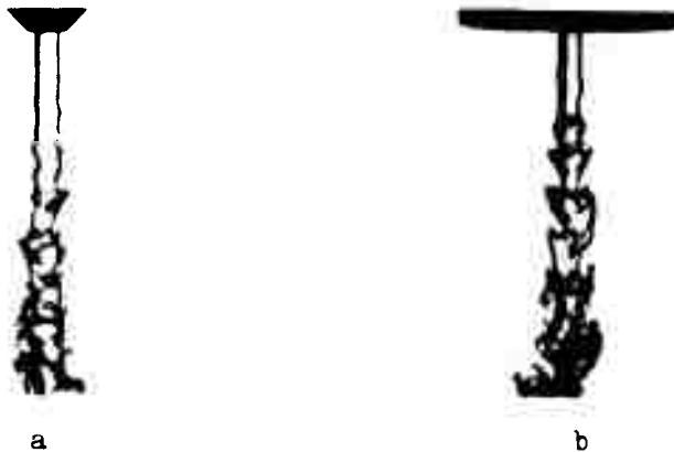
Fig. 11. Comparison of two jets emerging from a cylindrical and a contracted nozzle. Glycerine jet into water.
