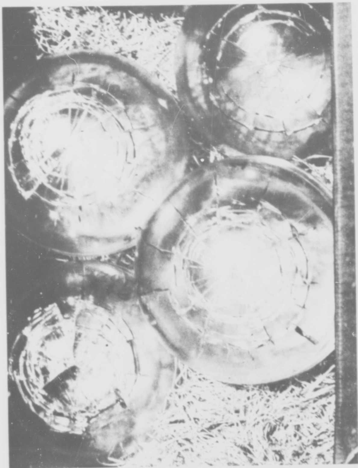
FIG. 3. TYPICAL COW MODEL DAMAGE AT 300 FT.
