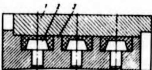
Fig. 12.17. Diagram of molding of rubber cups in a multiimpression mold.
