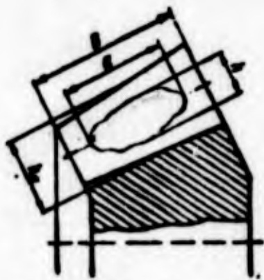
Fig. 5.45. Location of paint spot on the tooth of a gear.
