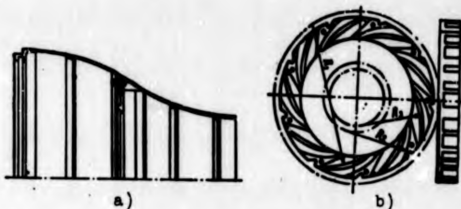
Fig. 8.3. Housing parts with shaped surfaces. a) welded diffuser; b) cast diffuser.
