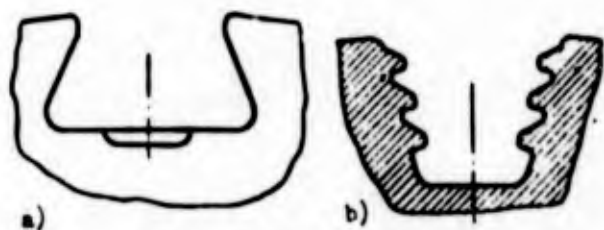
Fig. 2.2. Shape of grooves in compressor wheels. a) "Dovetail," b) fir-tree.
