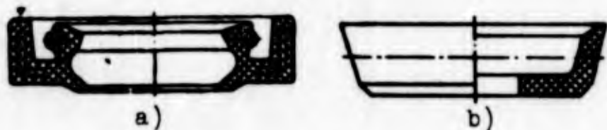
Fig. 12.8. Parts of packing. a) fitted sealing ring; b) cup without fittings.
