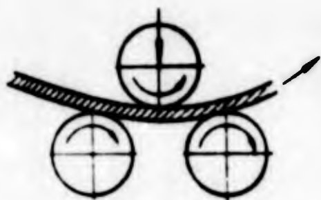
Fig. 7.15. Diagram of rolling on three-roller sheet-bender.
