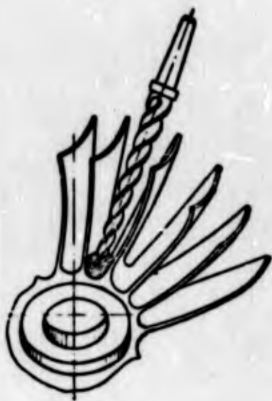
Fig. 4.13. Treatment of cavity base between vanes.
