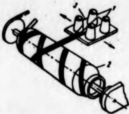
Fig. 12.9. Diagram of winding of a rocket engine housing by fiber glass. 1) coil with fiber glass; 2) mounting; 3) support.
