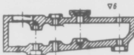
Fig. 8.17. Fine boring of holes in housing parts with parallel axes of holes.
